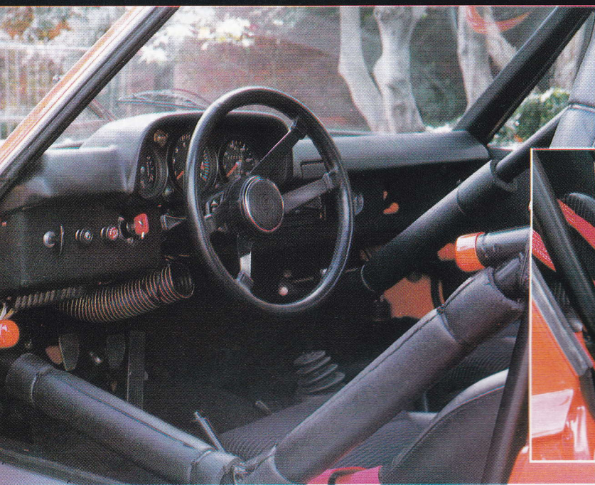
914-6 GT steering wheel was most difficult to locate. Updated dash panel uses generic factory race warning lights.
