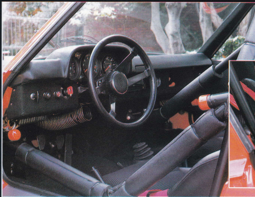
914-6 GT steering wheel was most difficult to locate. Updated dash panel uses generic factory race warning lights.
