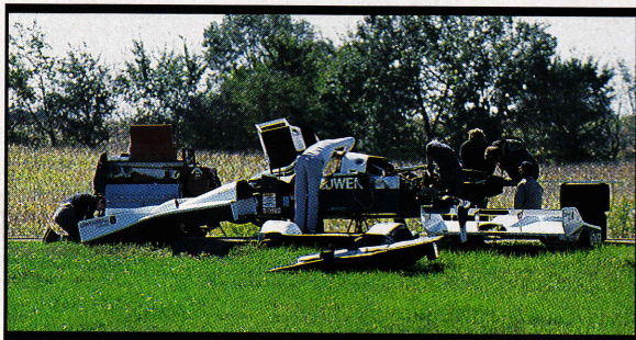
Installation of Le Mans tail and undertray enabled Porsche to achieve its best trap speed—227 mph.
