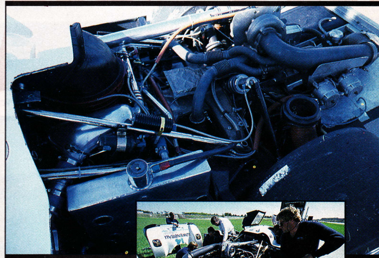
Study in contrasts: Space-capsule-like Porsche interior is chock-full of electronics, including dual Bosch Motronics that control operation of the 962's turbocharged flat-6. Stocker's roomy cockpit is model of simplicity as is the Chevy's carbureted stock block V-8.
