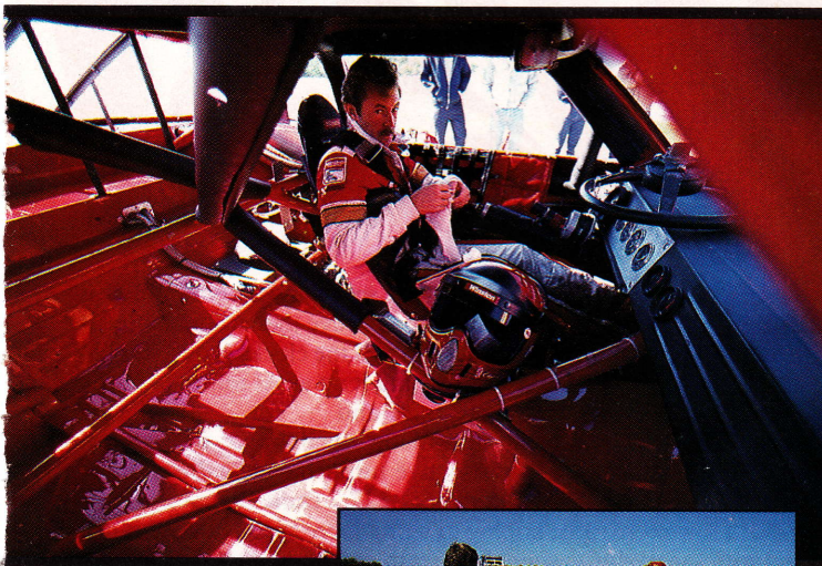
Study in contrasts: Space-capsule-like Porsche interior is chock-full of electronics, including dual Bosch Motronics that control operation of the 962's turbocharged flat-6. Stocker's roomy cockpit is model of simplicity as is the Chevy's carbureted stock block V-8.
