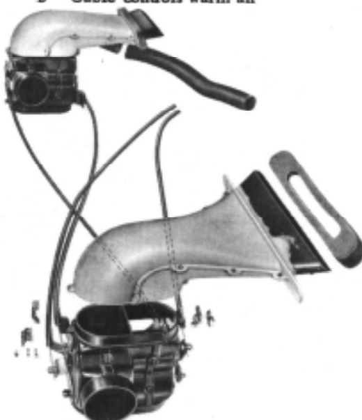
A - Cable controls fresh air B - Cable controls warm air
