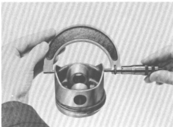
Fig. 7 Piston diameter (new) is stamped into the piston head. Measurements are made at the lower end of skirt, perpendicular to the piston pin axis.
