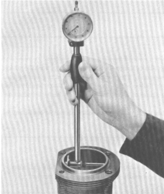
Fig. 6 Measure the cylinder bore approx. 10-15 mm below the top edge of cylinder.
