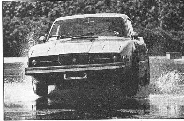
Understeering Saab was easiest to control in oil/wet skid pad.
