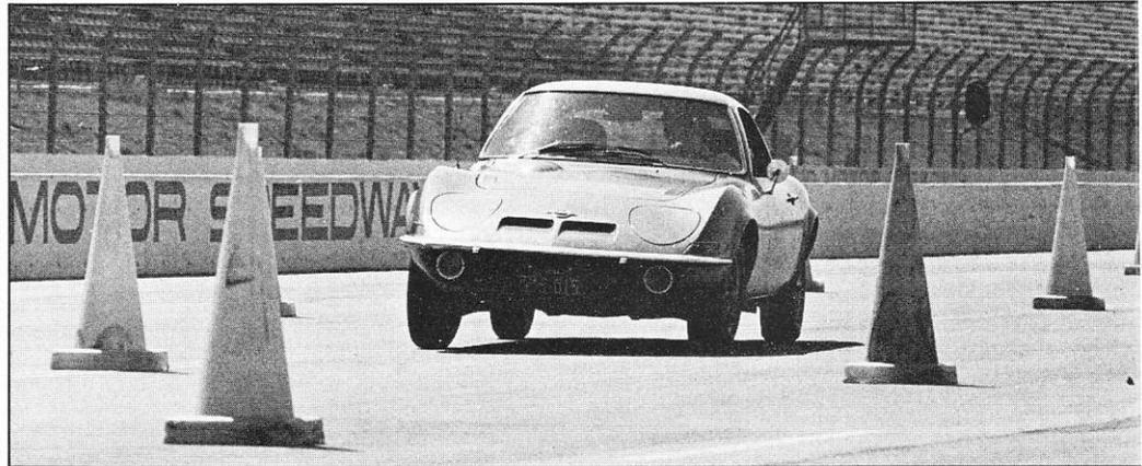
*Quick steering and the ability to hold a controlled power-on drift gained the front engine/rear drive Opel GT a second place in the lane-change maneuver.*
