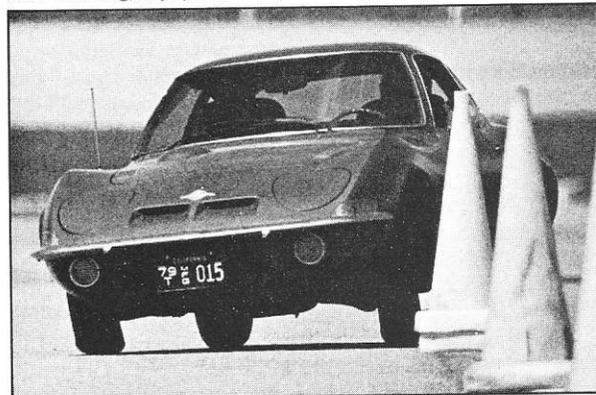
Heavily loaded outside front wheel worked against the Opel.
