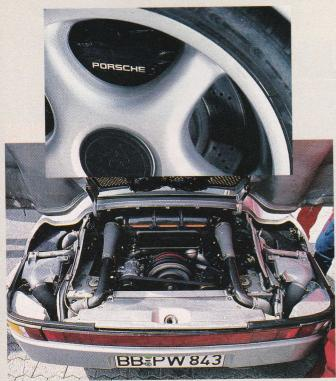
An exercise in symmetry: Twin intercoolers reside in flanks, twin turbos are inboard and beneath. Flat-6 produces 450 bhp DIN. And it's designed to run on European unleaded!
