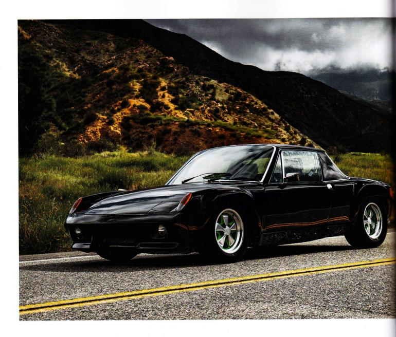
Although it resembles a 914/6 at first glance, Brutus wears unique bumpers with a front cutout for its trunk-mounted oil cooler. The bespoke Fuchs wheels are original; custom rubber was created for the restoration by Coker Tire and Michelin.
