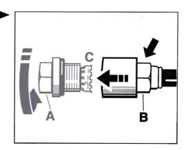
31. Insert the screwed plug into the plug-in coupling in a straight line. The plug must audibly engage in the holder.
