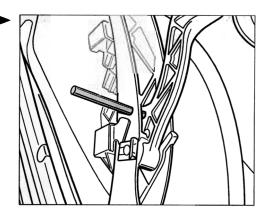
11. Open the rear wall cover. To do so, remove the oddments tray behind the seats and remove the rear wall lining. Then undo the 6 fastening screws and the 2 fastening nuts. (See -arrows-).
