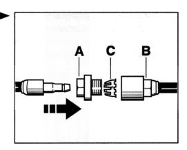
30. Insert the holder - C - into the threaded part -A - and screw both into the plug-in coupling - B - and tighten. Make sure to counter with a wrench when tightening. The tightening torque for the steering pressure line is 30 Nm (22 ftlb.) (wrench size 15). The tightening torque for the steering return line is 40 Nm (30 ftlb.) (wrench size 19).
