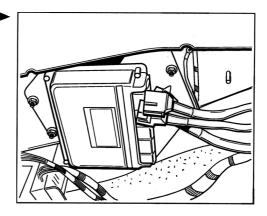
10. Connect the plug connections (X3/1, X3/2 and X59) of the engine wiring harness. To do so, insert the plug and lock the lateral slide.
