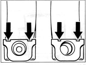
14. Turn crankcase by 180°. Make sure the bearing shell is correctly seated in the connecting rod. The fixing lugs point to the oil pan.
