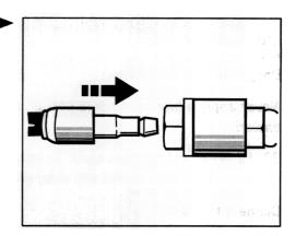
30. The correct engagement of the plug-in couplings should be checked using the special tool 9623. To check this, insert the special tool 9623 between the plug-in coupling and the screwed plug and tilt the tool slightly. The plug must not slide out.
