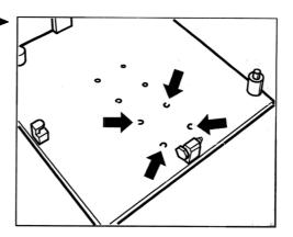
4. Fasten the special tool adapter 9163/2 with a hexagon-head bolt M8 x 25 (bolt quality 10.9) and hexagon-head bolts M8 x 16 (bolt quality 10.9) at the designated position "Boxster". The adapter and the support plate are fastened on the retainer plate with the M8 x 25 hexagon-head bolts. The M8 x 16 hexagon head bolts connect the adapter with the support plate.
