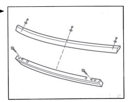
14. Remove rear bumper. While doing so, pay attention to the connection for the number plate lighting ⇒ 63; Rep. Gr. 63 58 19; Removing and installing rear bumper.
