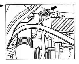
21. Fit the oil filler line. Push the oil filler line back onto the flange and secure with a spring band clamp.
