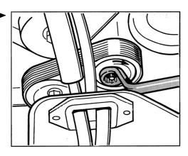
46. Undo the rear fastening screw of the air-conditioning compressor from above. The screw is positioned between the intake manifolds of the fifth and sixth cylinders.
