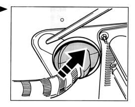
52. Disconnect the plug connection at the guide tube of the oil dipstick. To do so, press the two tabs together and unclip the tube.
