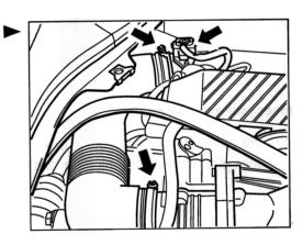
39. Press the spring band clamp on the oil filler hose apart and push it aside. Pull off the oil filler hose; heat, if necessary.
