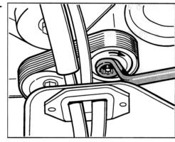
45. Undo the rear fastening screw of the air-conditioning compressor from above. The screw is positioned between the intake manifolds of the fifth and sixth cylinders.
