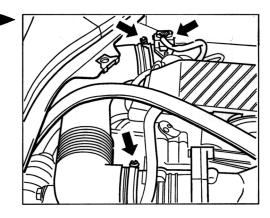
40. Press the spring band clamp on the oil filler hose apart and push it aside. Pull off the oil filler hose; heat, if necessary.
