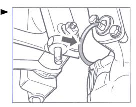
2. Push the engine wiring harness through the bulkhead and into the luggage compartment before the final installation position is reached.
