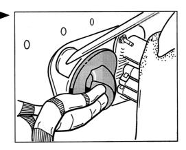
Re-connect engine control module. To do so, start at the bottom. Pay attention to the plug designations on the control module.
