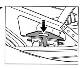
34. Unscrew the heat shield on the transmission. To do so, unscrew the two fastening nuts and remove the plate.
