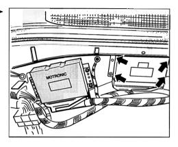
49. Disconnect control module. Disconnect the plugs of the Tiptronic control module. At the same time, lock the ground point of the engine control module.
