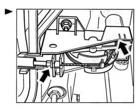
36. Disconnect the electric plug on the hot film mass air flow sensor. Then disconnect the connecting hose between the hot film mass air flow sensor and the throttle body. To do so, disconnect the hose clamp on the hot film mass air flow sensor.
