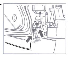
Remove the engine-transmission retainer plate. As soon as the I engine has been fastened again, the car jack and the retainer plate can be removed.
