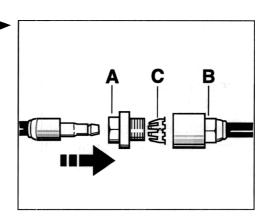
28. Insert the holder - C - into the threaded part -A - and screw both into the plug-in coupling - B - and tighten. Make sure to counter with a wrench when tightening. The tightening torque for the steering pressure line is 30 Nm (22 ftlb.) (wrench size 15). The tightening torque for the steering return line is 40 Nm (30 ftlb.) (wrench size 19).
