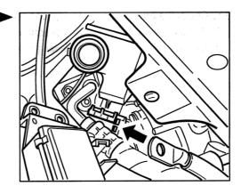
20. Re-connect hot film mass air flow meter. Connect the connect- ▶ ing tube between the hot film mass air flow meter and the intake system and tighten the hose clamp.
