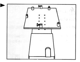
Engine retainer plate positioned and fastened.
