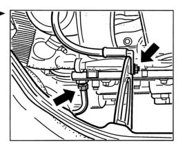
16. Push the vacuum line for the brake booster in a straight line on
