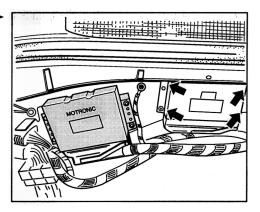
11. Connect the plug connections (X3/1, X3/2 and X59) of the engine wiring harness. To do so, insert the plug and lock the lateral slide.
