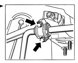
21. Unscrew the stabilizer on the left and right of the links.
