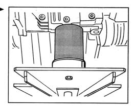
Clip the guide tube of the oil dipstick into the socket.
