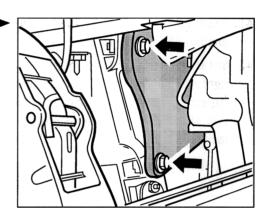
39. Move the exhaust system to its installation position again. In the process, replace all the seals at opened points. Tighten the three hexagon-head bolts again. Then tighten the screws on the exhaust manifold/catalytic converter with 25 Nm (18 ftlb.).
