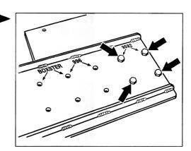
2. Countersink the retainer plate at the designated bores -arrows- with a 9 mm drill bit. The support plate serves as the drilling template.
