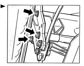
28. Remove the rear-axle support. Unscrew the four fastening screws and remove the rear-axle support to one side.
