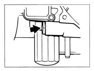
5. Loosen belt pulley. Undo hexagon-head bolt (M16 x 1.5 x 60) with special tool (socket wrench insert 9594); to do this, hold with holding device (special tool 9593).
