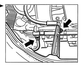
17. Push the vacuum line for the brake booster in a straight line on to the flange, until the plug is heard to engage. Then install the grey snap ring again. Check that the line is seated properly by pulling on it gently.
