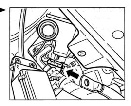
19. Re-connect hot film mass air flow meter. Connect the connecting tube between the hot film mass air flow meter and the intake system and tighten the hose clamp.
