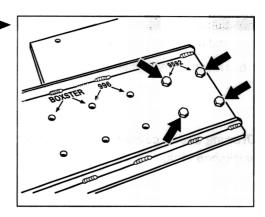
2. Countersink the retainer plate at the designated bores -arrows- with a 9 mm drill bit. The support plate serves as the drilling template.
