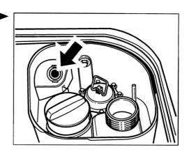
8. Fit the rubber sleeve of the wiring harness again.
