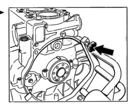
4. Insert the screwdriver in the lugs of the crankcase halves and separate the crankcase halves by tapping gently. Alternate the sides during separation.
