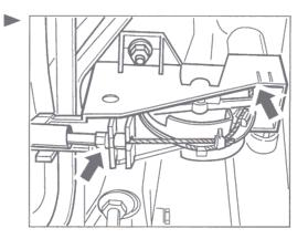
39. Disconnect the electric plug on the hot film mass air flow sensor. Then disconnect the connecting hose between the hot film mass air flow sensor and the throttle body. To do so, disconnect the hose clamp on the hot film mass air flow sensor.
