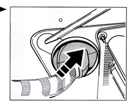
53. Disconnect the plug connection at the guide tube of the oil dipstick. To do so, press the two tabs together and unclip the tube.
