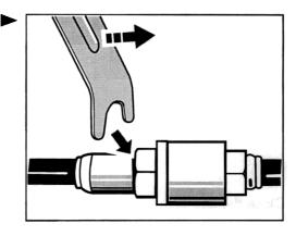
31. Install the servo lines, the return line and the vacuum hose for the brake booster again and insert the retaining clip.
