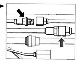
33. Disengage the retaining clips for the power-assisted steering lines and the brake vacuum hose and remove the lines.
