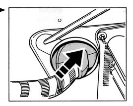
54. Disconnect the plug connection at the guide tube of the oil dipstick. To do so, press the two tabs together and unclip the tube.
