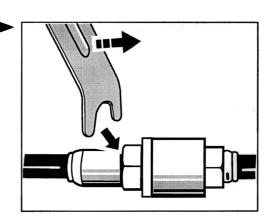
33. Install the servo lines, the return line and the vacuum hose for the brake booster again and insert the retaining clip.
