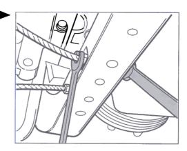
28. Connect the power-assisted steering lines. To do so, tilt the holder on one side and pull out simultaneously.
