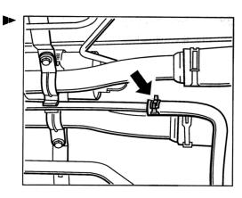
36. Install rear-axle support again. The four fastening screws are tightened to 65 Nm (48 ftlb.).
