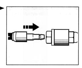
32. The correct engagement of the plug-in couplings should be checked using the special tool 9623. To check this, insert the special tool 9623 between the plug-in coupling and the screwed plug and tilt the tool slightly. The plug must not slide out.
