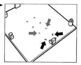
4. Fasten the special tool adapter 9163/2 with a hexagon-head bolt M8 x 25 (bolt quality 10.9) and hexagon-head bolts M8 x 16 (bolt quality 10.9) at the designated positions "Boxster". The adapter and the support plate are fastened on the retainer plate with the M8 x 25 hexagon-head bolts. The M8 x 16 hexagon head bolts connect the adapter with the support plate.
