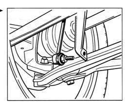
42. Install the sheetmetal brace into the vehicle. Tighten the hexagon nuts with 65 Nm (48 ftlb.) and tighten the fastening screws with 46 Nm (34 ftlb.). Install the two diagonal braces into the vehicle. Tighten the fastening nuts to 65 Nm (48 ftlb.).
