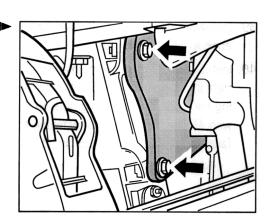
37. Move the exhaust system to its installation position again. In the process, replace all the seals at opened points. Tighten the three hexagon-head bolts again. Then tighten the screws on the exhaust manifold/catalytic converter with 25 Nm (18 ftlb.).
