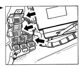
51. Lock the ground point of the engine control module.
