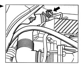
20. Fit the oil filler line. Push the oil filler line back onto the flange and secure with a spring band clamp.
