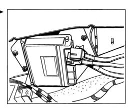
10. Connect the plug connections (X3/1, X3/2 and X59) of the engine wiring harness. To do so, insert the plug and lock the lateral slide.
