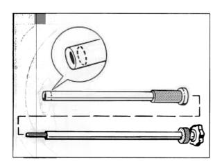
19.4 Carefully insert the pressure pin (1) of special tool 9602 into the assembly tube (2) until it contacts the piston pin circlip. The circlip can pop out of the assembly tube in the case of improper handling – danger of injury!
