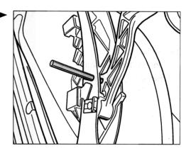
11. Open the rear wall cover. To do so, remove the oddments tray behind the seats and remove the rear wall lining. Then undo the 6 fastening screws and the 2 fastening nuts. (See -arrows-).
