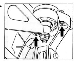
5. Install engine carrier again. Tighten the four fastening screws to 65 Nm (48 ftlb.).
