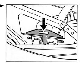
33. Disconnect plug from transmission socket. The plug must be turned anti-clockwise. Then pull off the plug.
