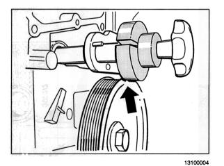
25. Move the piston pin circlip to its installation position by **briefly and forcefully striking** the palm of your hand against the star knob of the pressure pin.
