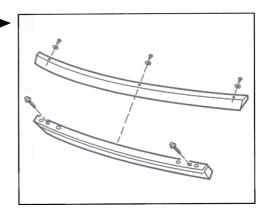
14. Remove rear bumper. While doing so, pay attention to the connection for the number plate lighting ⇒ Rep. Gr. 63 58 19; Removing and installing rear bumper.
