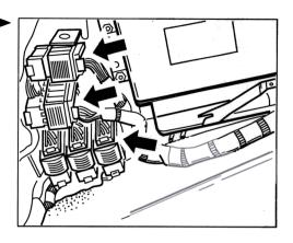
48. Remove the Tiptronic control module. Undo the three -fasten- ing nuts- and pull off the control module plug.
