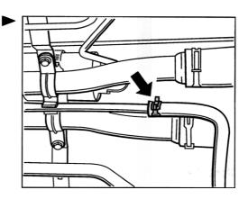
37. Install rear-axle support again. The four fastening screws are tightened to 65 Nm (48 ftlb.).
