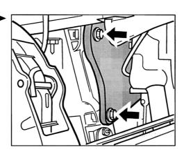
38. Move the exhaust system to its installation position again. In the process, replace all the seals at opened points. Tighten the three hexagon-head bolts again. Then tighten the screws on the exhaust manifold/catalytic converter with 25 Nm (18 ftlb.).
