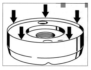
Illustration shows surrounding edge of centring piece. The surrounding edge must not be damaged.
