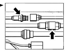
33. Disengage the retaining clips for the power-assisted steering lines and the brake vacuum hose and remove the lines.
