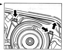
14. Check the drive belt for damage and replace it if necessary. Fit ▶ the belt in its original running direction once more. The fitting sequence is shown in the following illustration.
