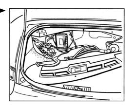
14. Screw air-conditioning compressor tight. Tighten the three fastening screws to 23 Nm (17 ftlb.).
