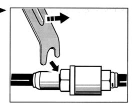
32. Install the servo lines, the return line and the vacuum hose for the brake booster again and insert the retaining clip.
