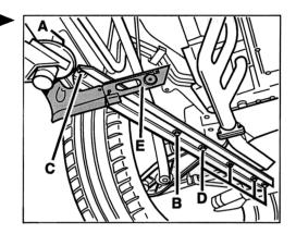
20. To do so, unscrew the two fastening screws at each of the two bearing surfaces on the left and right.
