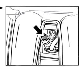
46. Loosen air-conditioning compressor. To do so, undo the two front fastening screws -(arrows)-. Disconnect the electrical plug.
