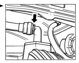
17. Install the expansion tank of the power steering again. Check the sealing rings and replace, if necessary. Turn the lower adjusting ring to its original position and position the tank of the power steering. Press the tank downwards and at the same time turn the ring until the markings coincide. Then fill the tank with Pentosin according to the regulations.
