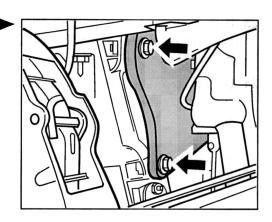
29. Drain coolant. To do so, remove the screw plug of the coolant circuit on the coolant guide housing. Collect coolant in a clean container.
