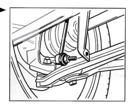
43. Install the sheetmetal brace into the vehicle. Tighten the hexagon nuts with 65 Nm (48 ftlb.) and tighten the fastening screws with 46 Nm (34 ftlb.). Install the two diagonal braces into the vehicle. Tighten the fastening nuts to 65 Nm (48 ftlb.).
