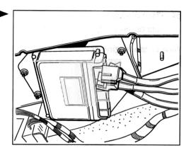
52. Uncover the engine wiring harness. To do so, press the rubber sleeve on the luggage compartment rear wall inwards and guide the wiring harness towards the engine compartment, if the engine is to be lowered later.
