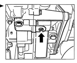
28. Disconnect coolant hoses. Open the supply and return lines for I coolant on the engine and pull them off. Then close all openings. Collect emerging coolant in a clean container.
