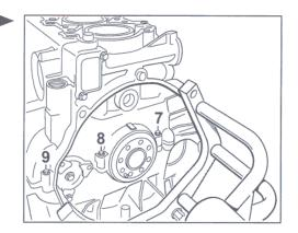
After tightening the crankcase halves, fasten the third fastening point between the crankcase half (cylinders 4 - 6) and special tool engine holder 9589.
