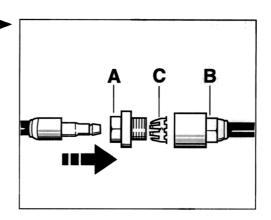
29. Insert the holder - C - into the threaded part -A - and screw both into the plug-in coupling - B - and tighten. Make sure to counter with a wrench when tightening. The tightening torque for the steering pressure line is 30 Nm (22 ftlb.) (wrench size 15). The tightening torque for the steering return line is 40 Nm (30 ftlb.) (wrench size 19).
