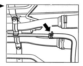
38. Install rear-axle support again. The four fastening screws are tightened to 65 Nm (48 ftlb.).
