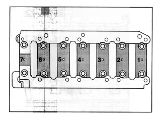
Arrangement of the connecting-rod bearings in the bearing housing.
