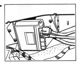
Re-connect and install the Tiptronic control module. Tighten the three fastening nuts.
