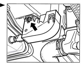
Disengage the accelerator cable
