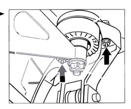
5. Install engine carrier again. Tighten the four fastening screws to 65 Nm (48 ftlb.).
