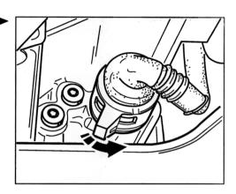
34. Detach selector lever cable at deflection linkage and at the transmission support.
