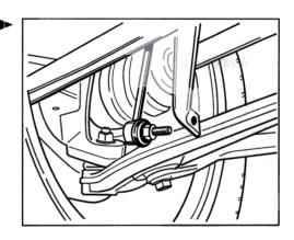
41. Install the sheetmetal brace into the vehicle. Tighten the hexagon nuts with 65 Nm (48 ftlb.) and tighten the fastening screws with 46 Nm (34 ftlb.). Install the two diagonal braces into the vehicle. Tighten the fastening nuts to 65 Nm (48 ftlb.).
