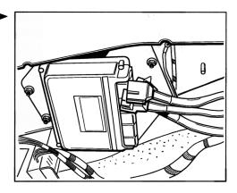
53. Uncover the engine wiring harness. To do so, press the rubber ► sleeve on the luggage compartment rear wall inwards and guide the wiring harness towards the engine compartment, if the engine is to be lowered later.
