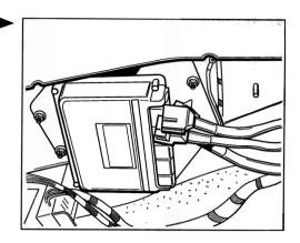
51. Uncover the engine wiring harness. To do so, press the rubber
