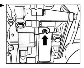
30. Disconnect coolant hoses. Open the supply and return lines for a coolant on the engine and pull them off. Then close all openings. Collect emerging coolant in a clean container.
