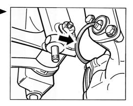
2. Push the engine wiring harness through the bulkhead and into the luggage compartment before the final installation position is reached.
