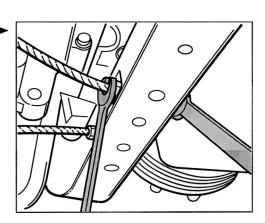
27. Connect the power-assisted steering lines. To do so, tilt the holder on one side and pull out simultaneously.
