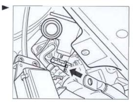
19. Re-connect hot film mass air flow meter. Connect the connect- I ing tube between the hot film mass air flow meter and the intake system and tighten the hose clamp.
