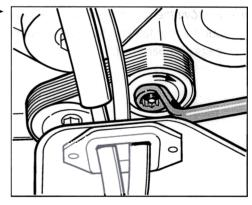
43. Undo the rear fastening screw of the air-conditioning compressor from above. The screw is positioned between the intake manifolds of the fifth and sixth cylinders.
