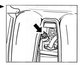
44. Loosen air-conditioning compressor. To do so, undo the two front fastening screws -(arrows)-. Disconnect the electrical plug.
