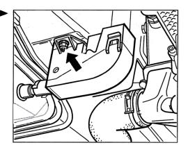
23. Engage selector lever cable at deflection lever and at the transmission support.
