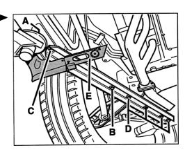
20. To do so, unscrew the two fastening screws at each of the two bearing surfaces on the left and right.
