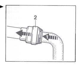
41. Remove supply tank of the power steering system. To do so, suck fluid out as much as possible. Then open the bayonet lock on the bottom of the expansion tank and remove the tank. Close the opening in the servo pump with a clean plug.
