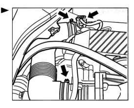
37. Press the spring band clamp on the oil filler hose apart and push it aside. Pull off the oil filler hose; heat, if necessary.
