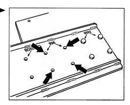
3. Drill through the countersunk bores on the retainer plate with a drill bit sized 6.8 mm and then cut an M8 thread.
