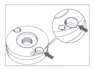
Illustration shows rounded edges on the 13590005 recesses in the centring piece.
