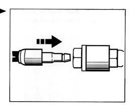
31. The correct engagement of the plug-in couplings should be checked using the special tool 9623. To check this, insert the special tool 9623 between the plug-in coupling and the screwed plug and tilt the tool slightly. The plug must not slide out.
