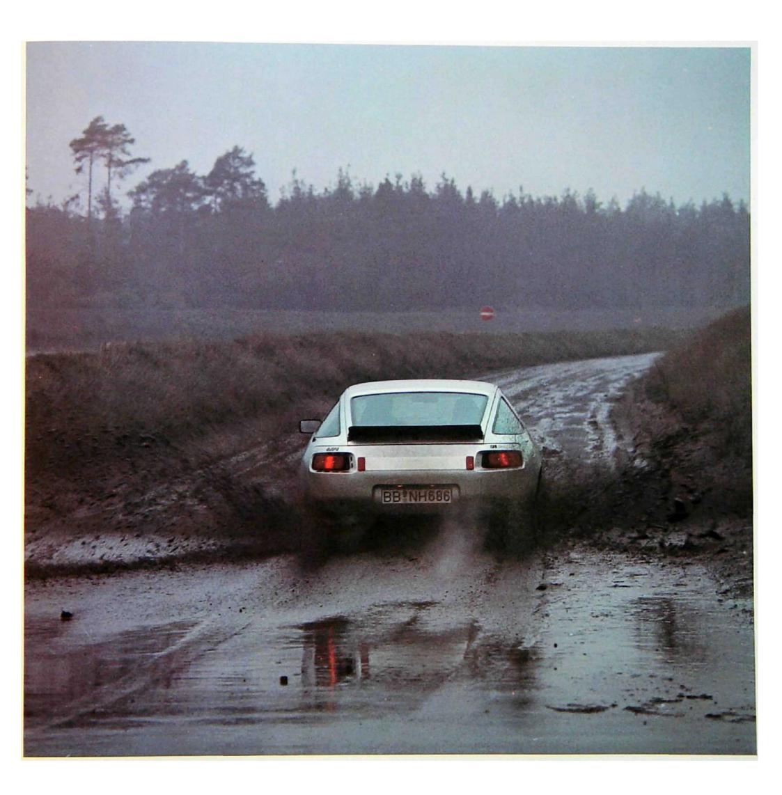
The test program included extreme water splashes to confirm sealing of the ignition system and body, as well as to check on aquaplaning reactions. The photos, left and right, show a vehicle before and during its passage through a flooded corner. They are checking aquaplaning behavior in a curve. Bottom and right side; passing through the deep water splash.
