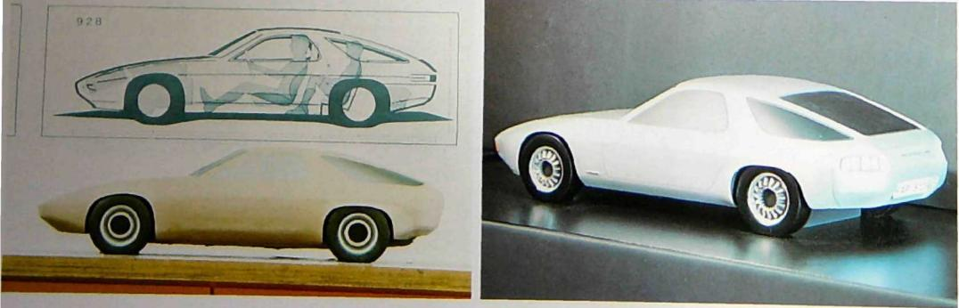
The first wind tunnel models were tested in the winter of 1971/72. During these tests various temporary modifications were applied which gave the models a very "provisional" appearance. The pictures show versions with nose spoilers and various tail layouts.
