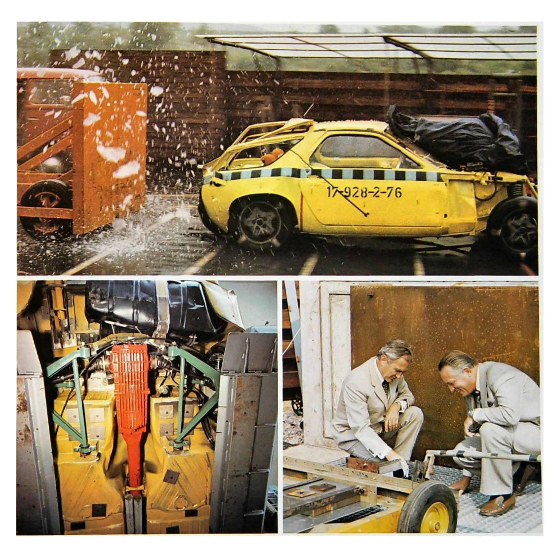
Frontal crash with dummies in the vehicle and a speed of 30 mph. Here too the result was more than convincing: deformation of the nose section came at predetermined points, the passenger cell was undamaged in the crash and the doors didn't spring open.
