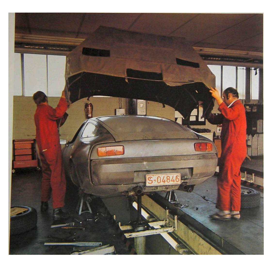
Test beds that one doesn't see every day: a 928 body on the rig to measure torsional body stiffness and a test rig for elasticity measurement on the front axle (bottom).
