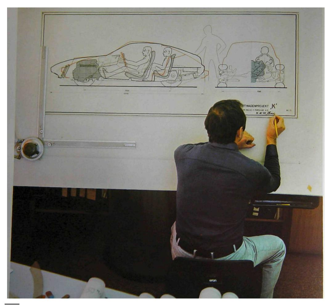
Selected project designs are based on examination and evaluation of countless pre-designs. Such sketches (left: suggestions for fitting aggregates into the tail area) give designers a necessary over view of the values for various spatial dispositions. Design boss Wolfgang Eyb (bottom) also played an intensive role in the search for optimum arrangement for all aggregates.
