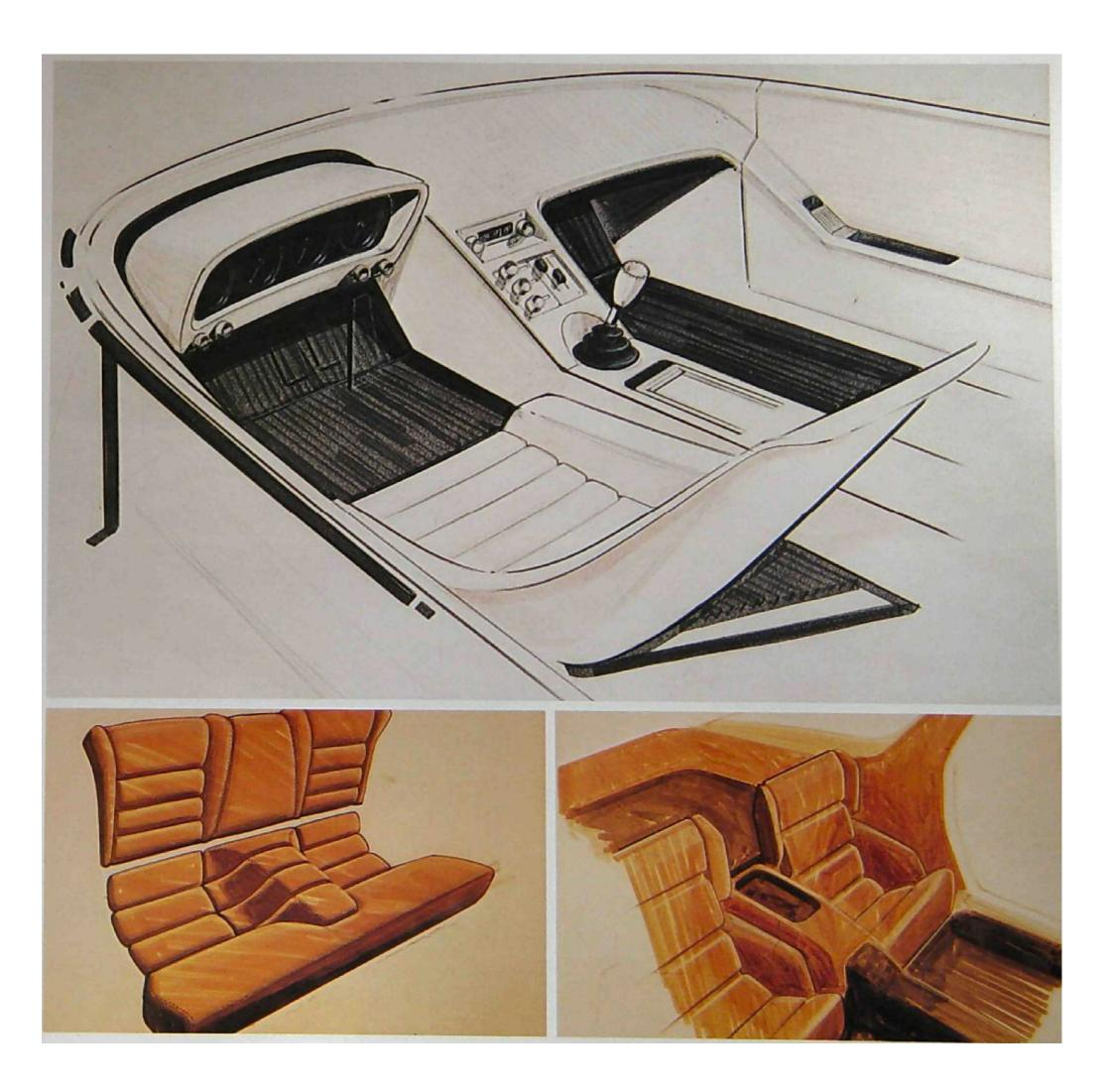
The skeleton model or seating buck was completed in the spring of 1972 and became an indispensable tool. Effective space relationships could be evaluated with its aid as they resulted from predetermined dimensions and styling studies.
