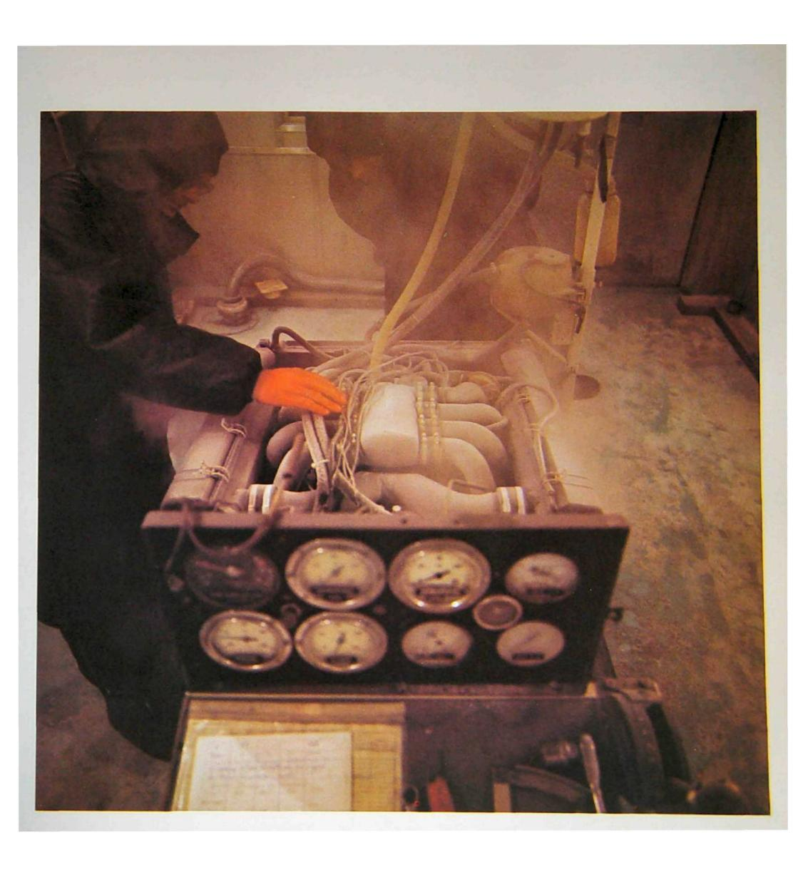
In 1972, as pre-testing was getting underway, Chassis Testing outfitted the first mobile test bed. Left; V I, a Mercedes 350 SL with original engine. The first transaxle experiments were carried out on this car. Later V I was fitted with a 928 carburetor engine (right).
