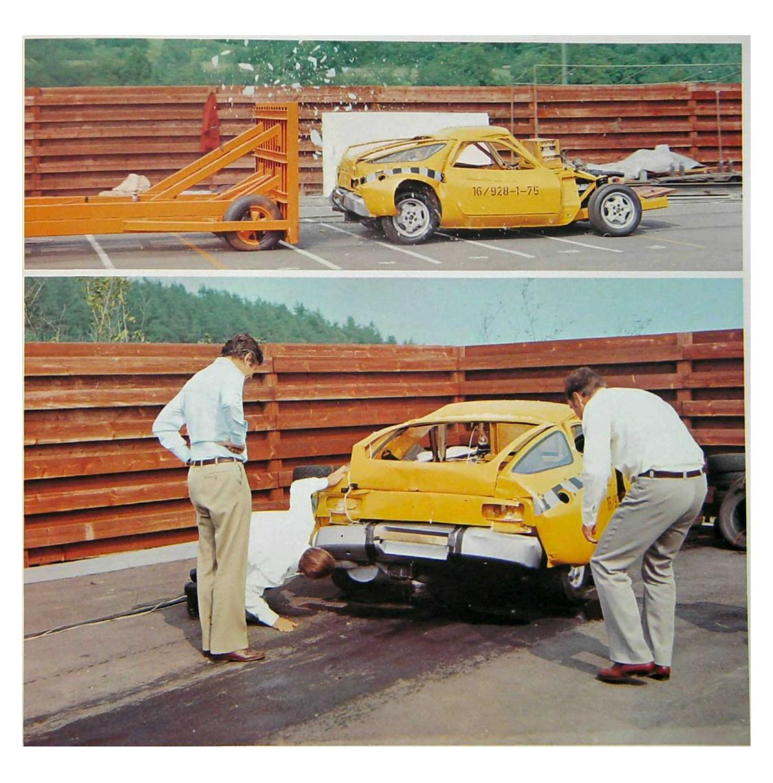
Repeat of the same rear crash test with modifications for better tank protection (still a sheet steel version here) and with integrated bumpers. Dr. Ernst Fuhrmann and Helmuth Bott register satisfaction at the progress - tail deformation met all projections and the tank remained tight.
