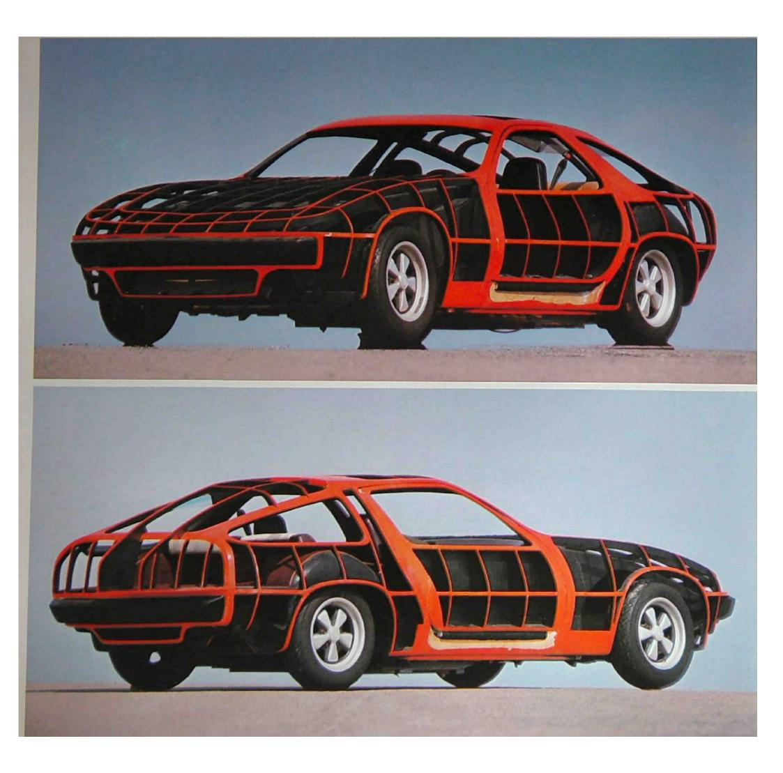
Measurements were taken from this buck during the early summer of 1972 on the grounds of the Weissach test track. Project Director Wolfhelm Gorissen (sitting on the model's tail, below) and his; co-workers check interior dimensions, entry conditions, view conditions and scaling comfort for driver and passengers.
