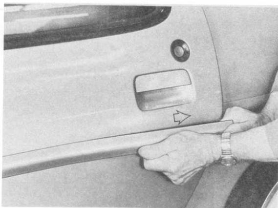
3. Used side guard strips can be used again, if the old adhesive strips are pulled off and new double-sided adhesive foam rubber strips are installed (3 M, Art. No. 4262, 19 mm wide). The primed adhesive surface of the strip must not be washed!
