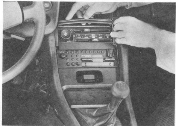
12. Insert lower mask frame with digital clock and connect digital clock.
