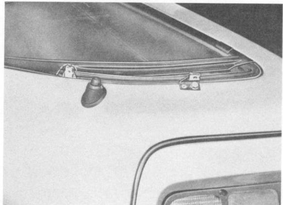
2. Mount seal on inner frame. Mount bracket on inner frame with M 6 x 16 oval head screw and on spoiler with M 6 x 10 hex. head screw with washer.
