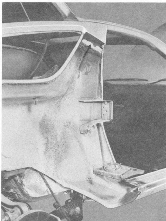
11. Solder welded seams on rail, door frame, lid frame and fender end section, and prepare them for painting.
