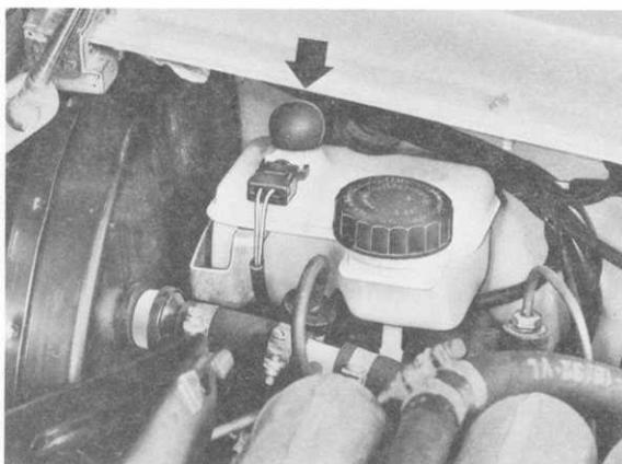
CWL, ABL and brake fluid IL should start to flash after approx. 20 seconds.
