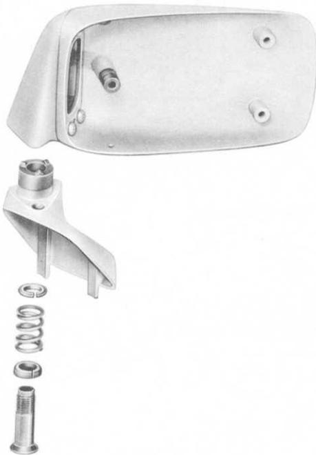
5. Push threaded insert into door reinforcement and hold with a rollpin.
