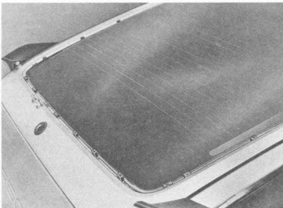
3. Install rear spoiler. Mount with 4.2 x 32 mm metal screws and washers. Watch for neat fit on lid. Use two M 4 nuts and above mentioned washers at upper part.
