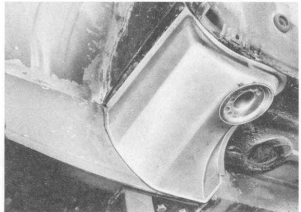
11. Position console for stabilizer on side member (295 mm from front cross member bolt, rear edge vertical) and weld to side member.
