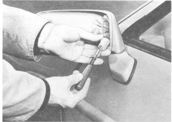
4. Unscrew fillister head screw on mirror base so that mirror can be removed with the liner.
