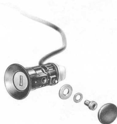
Doors with the new mounting point and new door lock cylinder require a spacer, 6.4 mm dia. washer, and a M 6 x 18 mm fillister head screw.
