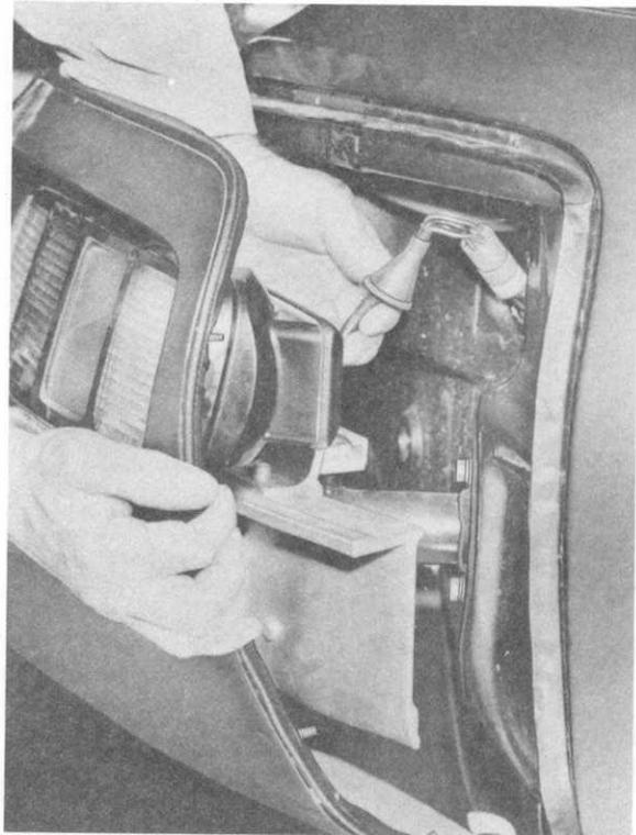
2. Until introduction of new PU panels, a weatherstrip has to be pasted on the mating surfaces to the rear side panels and fastened with clips. In this manner small irregularities in the body contour can be equalized or covered up.
