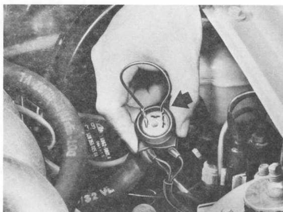
CWL, ABL and brake circuit IL must flash. Press acknowledgement button. All lamps should continue to flash. Disconnect bridge and connect plug on stop light switch. Lamps should continue to flash.
