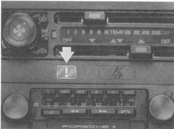
The central warning unit contains a "bulb check" function to check the light bulbs. All indicator lamps, the central warning lamp and the acknowledgement button lamp must come on after turning on the ignition.
