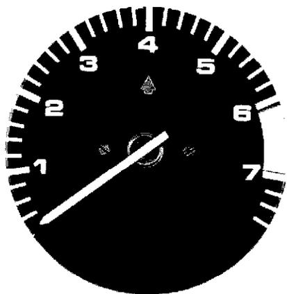
The upshift indicator will light up when it is practical and economical to shift up into the next higher gear. It works in gears 1 through 4 and remains illuminated until the next higher gear is engaged or the operating condition causing illumination of the indicator is changed (e.g. coasting, full throttle, etc.).
