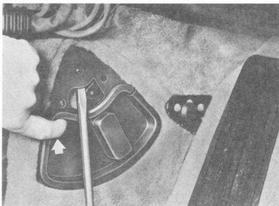
7. Remove cable grip and lay aside. Drive out spiral pin and pull hood cable with protective sleeve forward out of the housing.
