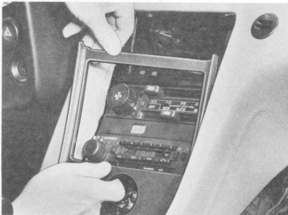
4. Unscrew tray underneath glove box and trim on side of center console.
