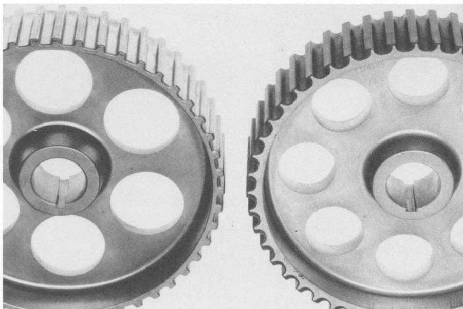
Note: New HTD drive belts can also be used on older engines, if above mentioned sprockets with new tooth shape are used at same time.
