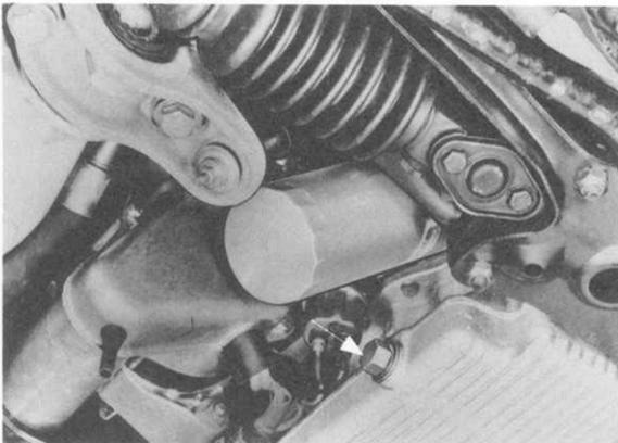
3. Loosen oil filter with a standard strap wrench, or US 4462.
