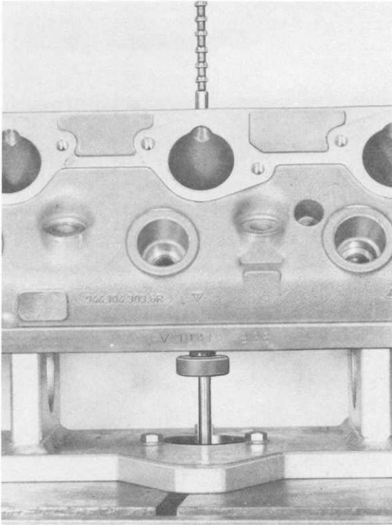
10. Valve seat inserts must be machined after replacing valve guides. Grinding in valves with grinding paste will not be sufficient.
