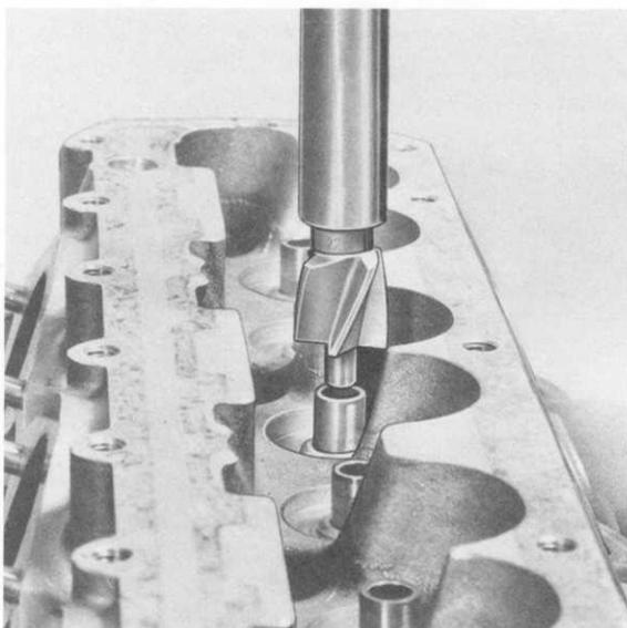
4. Loosen valve guides from camshaft end with brief hammer knocks on Special Tool 9224 and press out rest of guides toward combustion side with a press.
