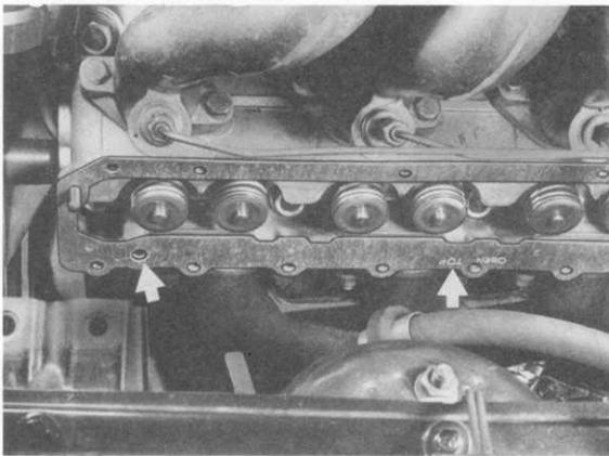
Note installed position of camshaft housing gasket. Camshaft oil bore must be clear (arrow).
