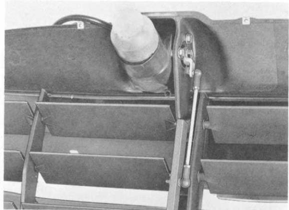
If the flap positioning motor fails to assume one of the positions stated, use an ohmmeter to check the conductivity of the control unit - flap positioning motor wire harness.
