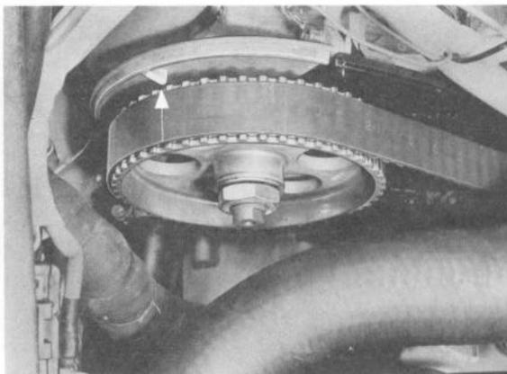
3. Unscrew drive belt guard upper section on both sides and remove.
