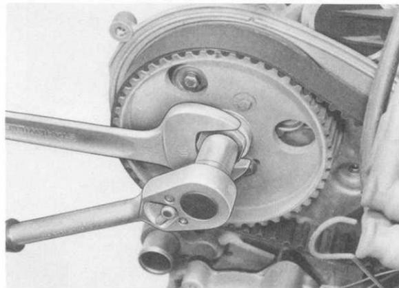
CHECKING AND ADJUSTING CAMSHAFT
