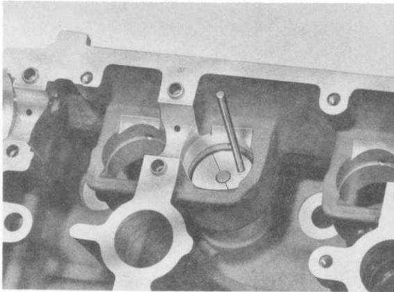
4. Do not mix up the valves after adjustment.
