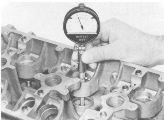
5. Machine KD valve guide, part no. 944 104 327 51 (external diameter 11.26 mm) to correct size.
