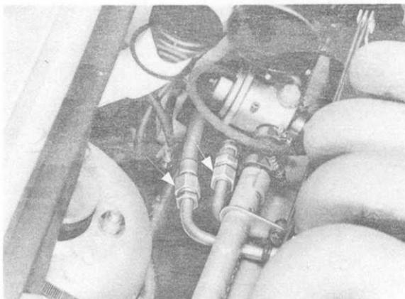
46. Detach hydraulic line at power steering pump.
