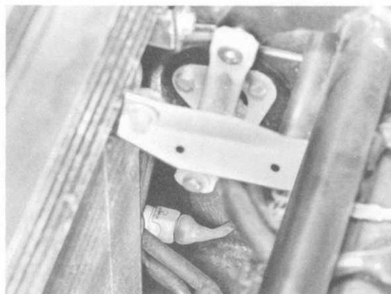
Tightening torque: 30 Nm (22 ft1b)
