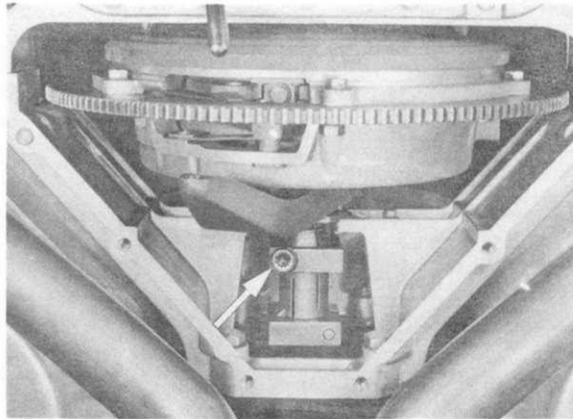
24. Unscrew throwout bearing sleeve mounting bolts and push sleeve in direction of clutch.
