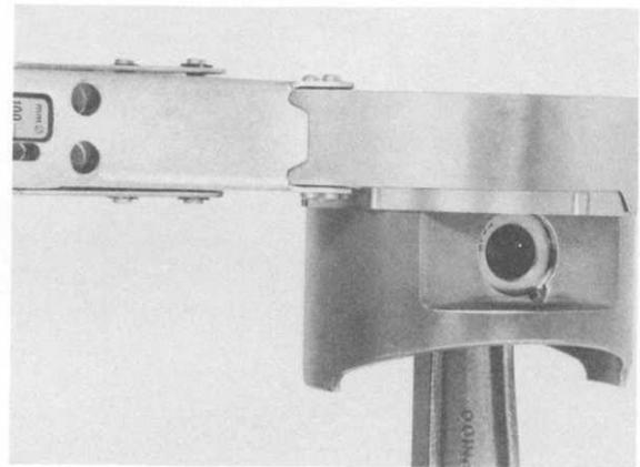
5. Install piston with connecting rod in cylinder bore and knock into cylinder by applying light knocks from hammer's handle and applying firm pressure to edge of compressor.
