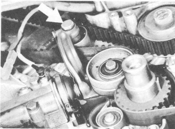
19. Remove toothed-belt from right-hand side over cylinder 1 - 4 camshaft sprocket, water-pump sprocket, cylinder 5 - 8 camshaft sprocket, oil-pump sprocket and crankshaft sprocket.
