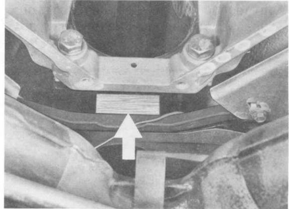
47. Tilt engine carefully toward front, lifting slightly. Once engine housing and clutch housing separate, engine can be hoisted out of vehicle.
