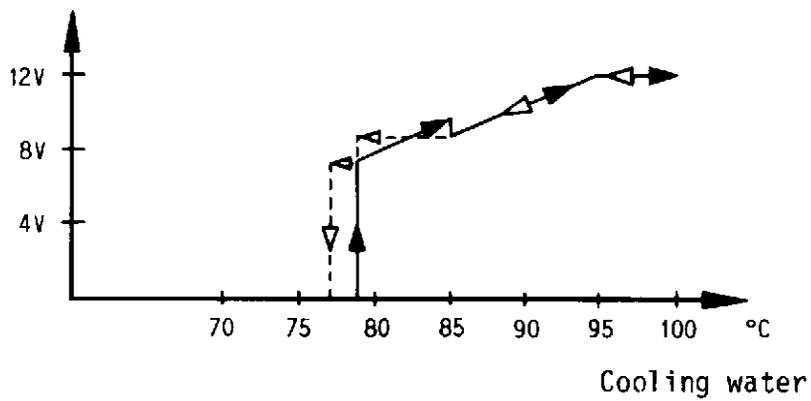
Temperature switch, automatic transmission
