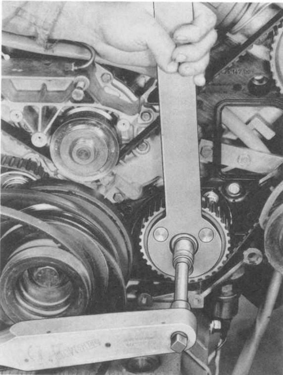
2. Unscrew the oil pump mounting bolts and remove oil pump.
