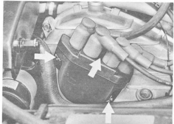
7. Take off both distributor rotors. Disconnect plugs for A/C compressor and toothed belt tightness indicator.
