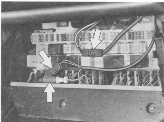
42. Disconnect multiplugs from EZF and LH control units, together with multiplug at right of central electrics unit.
