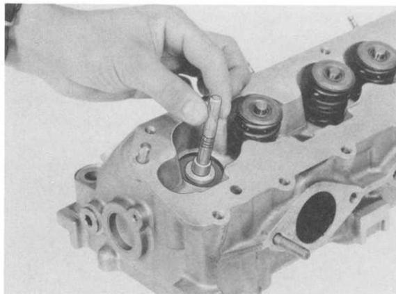
Lubricate valve stem seal and push on to valve guide carefully with the pressure pad.
