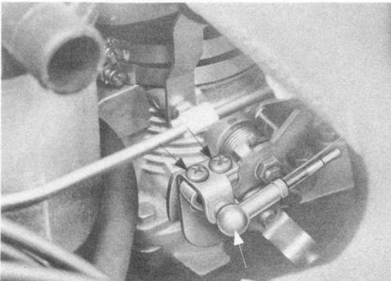
51. Engage adapter 9137 (in conjunction with floor hoist) in the eyelets provided for this purpose. Raise adapter until tight on engine.
