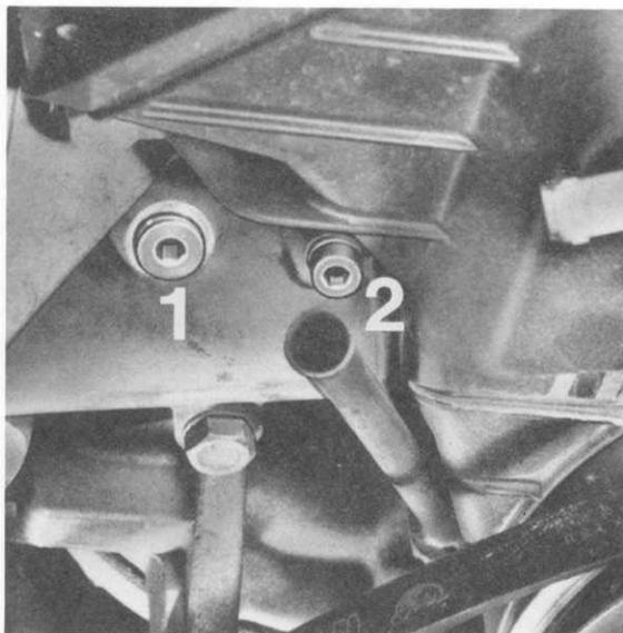
3. Pour oil from oil can into oil filler opening, slowly, until oil runs out of bleeder screw bore.
