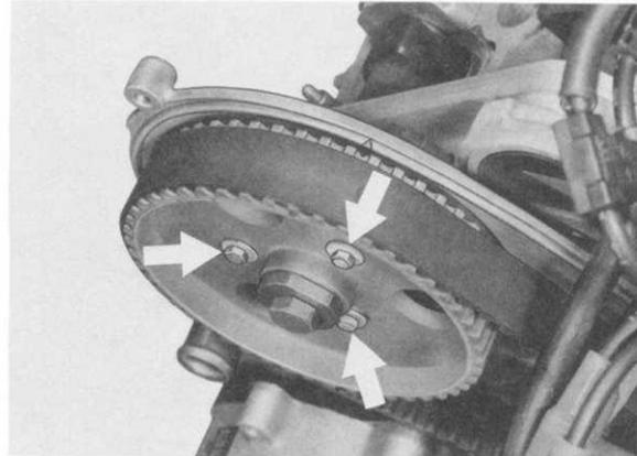
2. Turn crankshaft in its usual direction of rotation until the gauge shows a lift of  $1.6 \pm 0.1$  mm.
