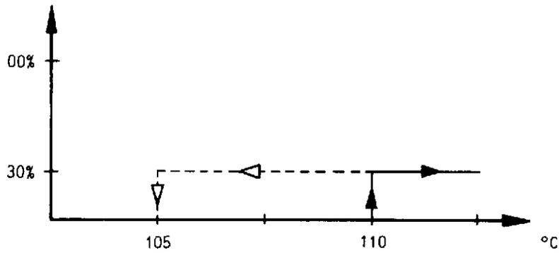
Temperature switch, automatic transmission
