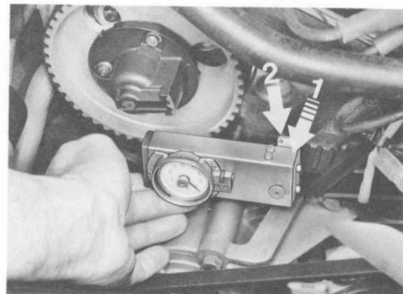
Read test value without tension in tester, i.e. tester must be kept horizontal to the toothed belt. Tester must not rest on the plastic cover.
