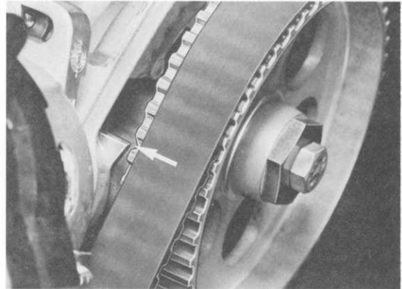
3. Turn engine two more turns until TDC mark is reached again and check drive belt for damage and wear at the same time.
