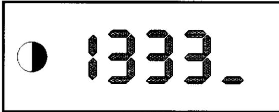
Press the accelerator pedal down slowly until the full load position has been reached. At the same time, the LED must go out and the following display will appear.
