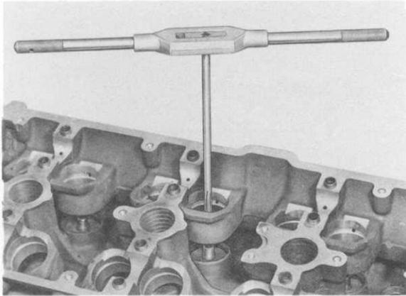
8. The valve-seat rings must be remachined when the valve guides have been replaced. It is not sufficient to grind in the valves with grinding paste.
