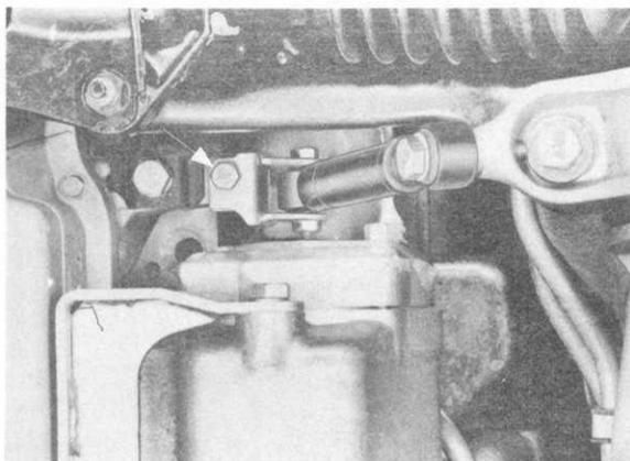
28. Loosen compressor, remove from console and suspend it with the hoses connected.
