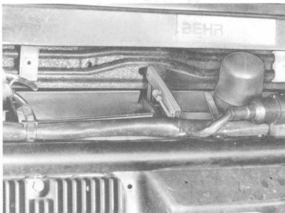
The control unit for the flaps and cooling-air control is positioned beside the passenger seat.
