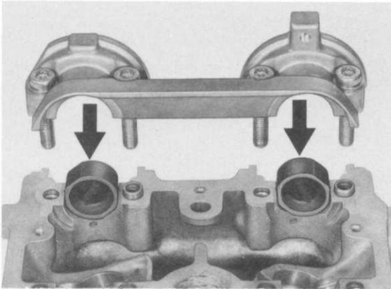
2. After torquing the bearing bridge, install sealing cover with the aid of Special Tool 9234.
