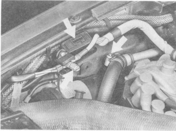
33. Disconnect bleed hose from cooling water expansion tank at engine and remove.
