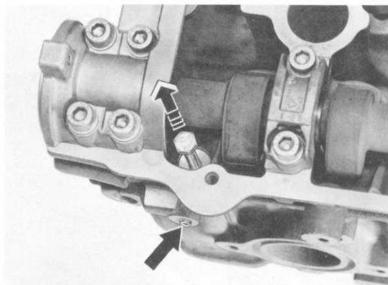
2. Use a magnet to withdraw compression spring and ball. Thoroughly clean ball seat, ball, compression spring and oil duct. The ball seat remains in the cylinder head and great care must be taken to ensure that it is not damaged.
