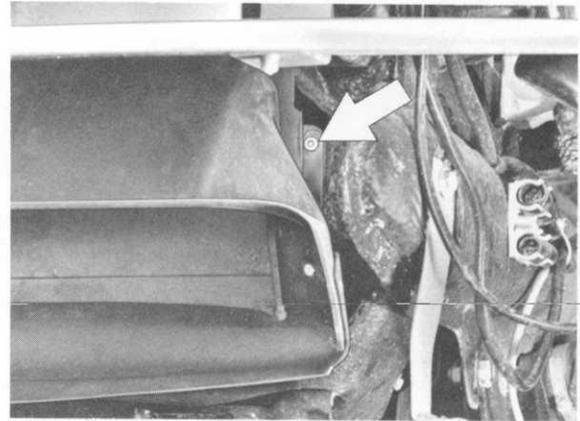
Disconnect plug of flap positioning motor at coupling.
