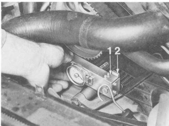
Line up maximum indicator with gauge indicator (in anticlockwise direction).
