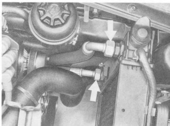
30. Disconnect cable from temperature switch at bottom left of cooler.
