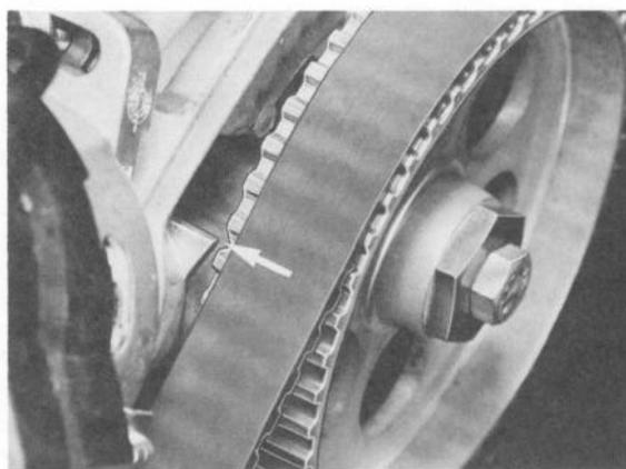
4. Turn engine in direction of rotation to TDC (cylinder 1). In this position marks on camshaft sprockets should conform with marks on flange bearings.
