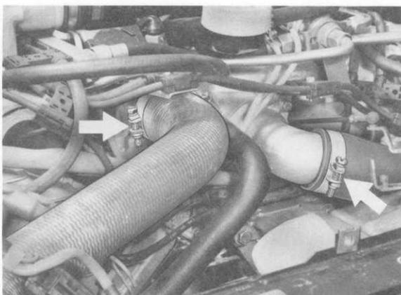
29. Detach oil hoses for engine cooling and ATF cooling from top and bottom of cooler, countering with second open-ended wrench.
