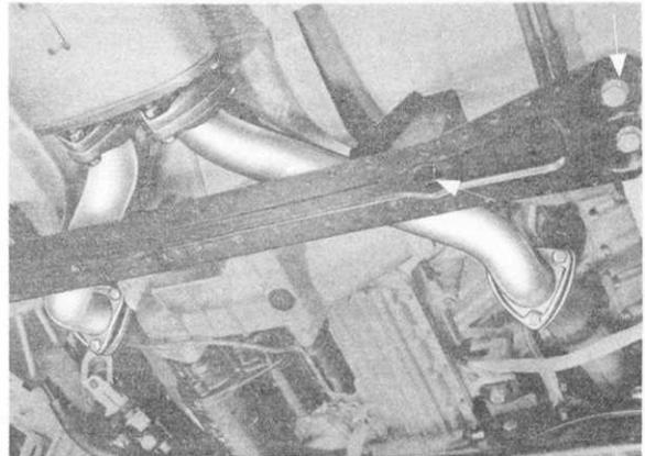
14. Detach exhaust pipes at exhaust manifolds and heat shields on left and right sides.
