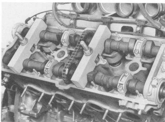
13. Release special tool uniformly and remove both camshafts with chain carefully.
