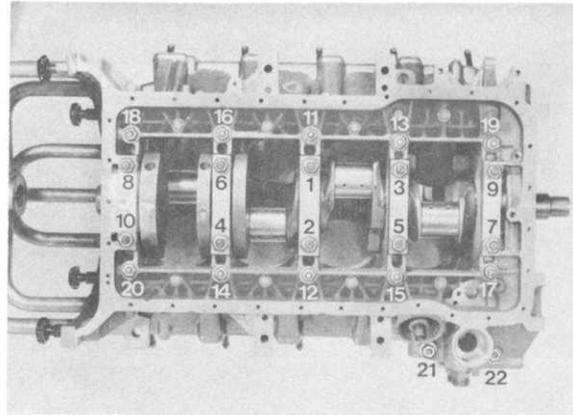
6. Mount upper section on engine holder after tightening nuts.
