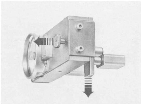
7. Slide special tool on to relaxed section of drive belt (sliding shoes on smooth surface, rollers in tooth gap).
