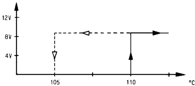
Temperature switch, automatic transmission
