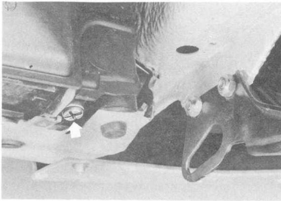
4. Unscrew coolant drain plugs on left and right-hand sides of crankcase and catch coolant.
