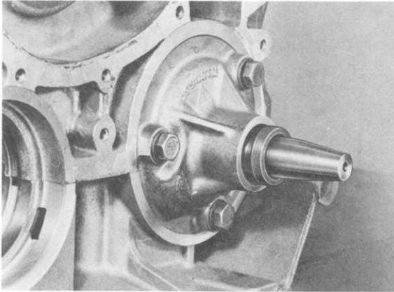
2. Knock in seal flush with a suitable pressure pad, e. g. VW 420.
