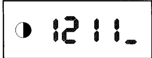
The error is displayed until the *green* key is pressed again on the tester. The next error code is then displayed, if applicable.
