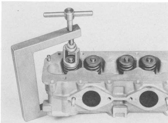
Remove and install valve springs with P 200 a.
