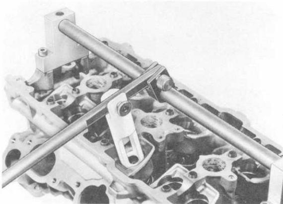
4. Use the magnetic disassembly head to withdraw all the valve spring parts.
