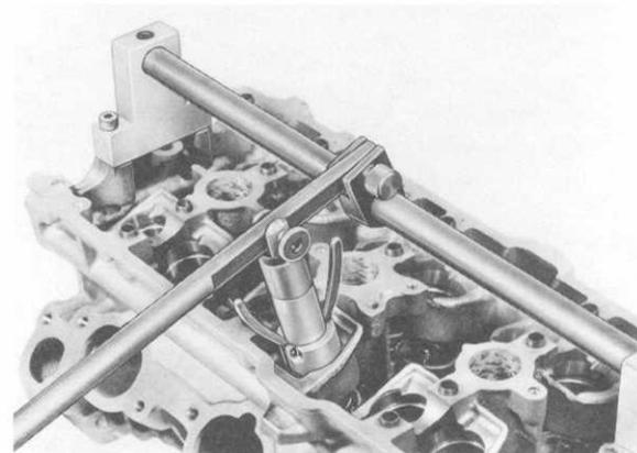
7. When the taper valve keepers are engaged, the clamping arms of the assembly head point out.
