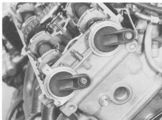
10. Set marks on camshafts to face up by turning exhaust camshaft with a 27 mm open - end wrench.
