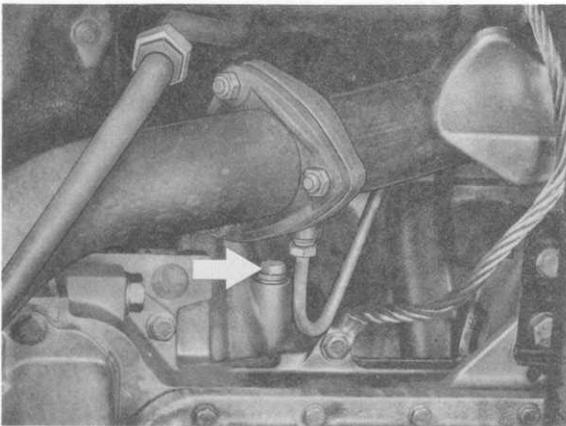
12. Drain engine oil. (Only if engine is to be overhauled.)
