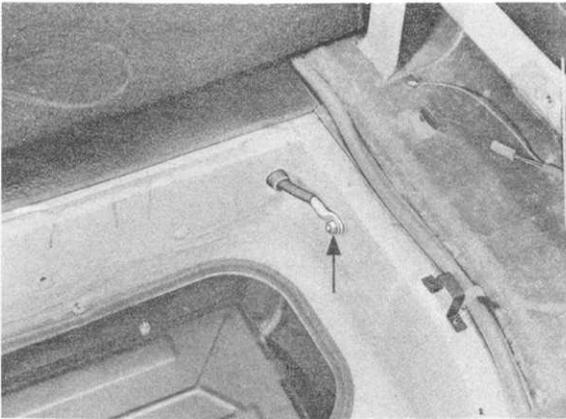
3. Loosen and remove engine compartment cross brace.
