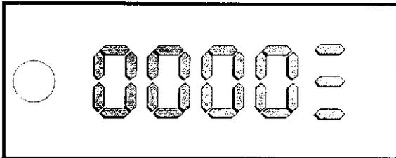
Press the *green* key until the clear symbol appears on the function display. Start the engine within 8 seconds. Allow the engine to idle until the system adaption code appears.
