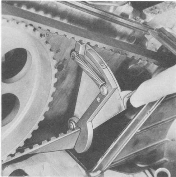
5. Turn engine clockwise two turns to align red indicator and TDC mark.
