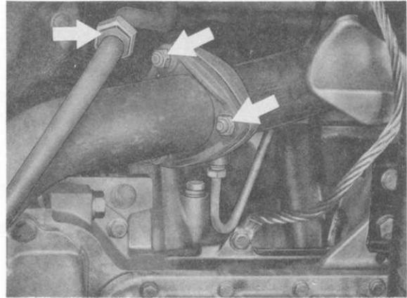
14. Disconnect body-engine ground connection at engine.
