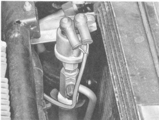
Tightening torque: 30 Nm (22 ftlb)
