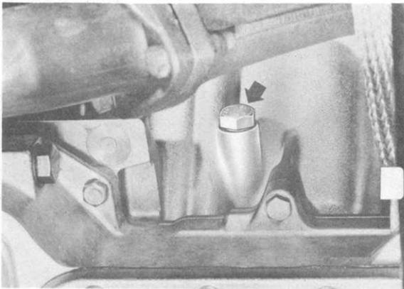
5. Replace seals for drain plugs on crankcase and O-ring for drain plug on radiator.
