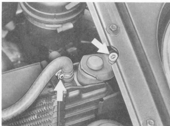
32. Disconnect coolant filler hose from cooler tube at front right, and remove. Disconnect multi-plug and B+ terminal.
