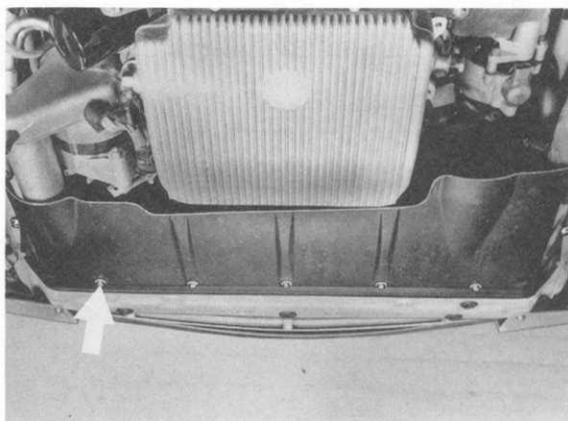
10. Drain cooler. (Catch coolant in suitable container).
