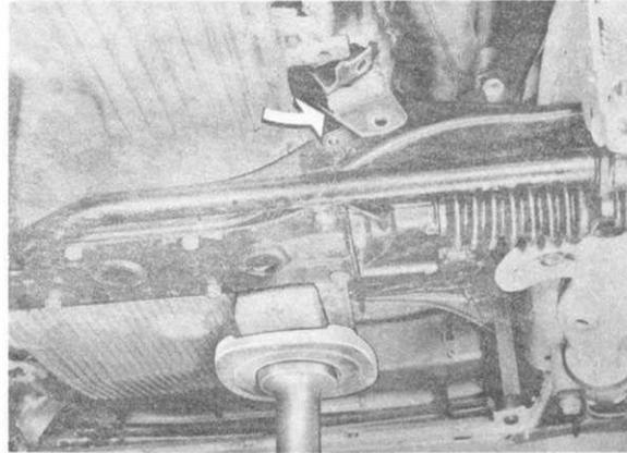
35. Remove clutch/engine mounting bolts.
