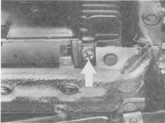
11. Unscrew water drain plugs on left and right of crankcase upper half.
