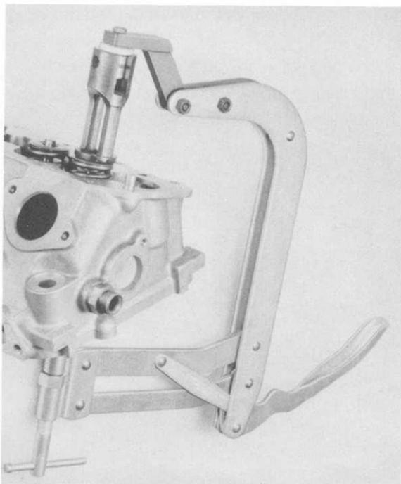
Remove and install valve springs with US 1020 (only applicable for USA).
