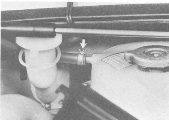
2. Connect tester VW 1274 with separate T-adapter and pertinent hoses ahead of the expansion tank.
