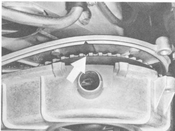
8. Slide special tool on released belt section of toothed belt (sliding shoe on smooth surface, roller must fit in tooth gap).
