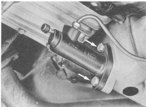
2. Guide in special tool and mount with standard bolts.
