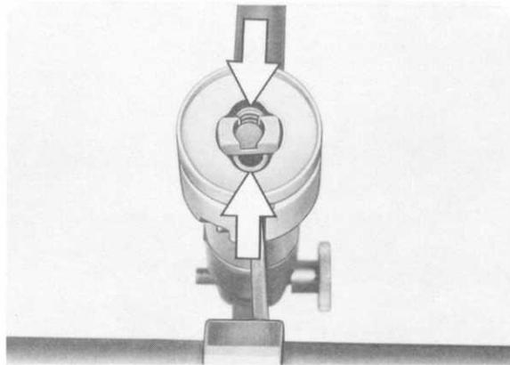
6. Place washer, valve spring stop, valve spring and valve spring plate in cylinder head and compress with assembly head. Engage taper valve keepers by moving lever up and down slightly. This action automatically positions the taper valve keepers correctly.
