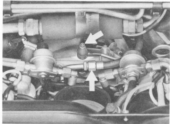
24. Disconnect hose from heating regulator and pipe stub on engine and remove. Pull underpressure line for automatic transmission from underpressure distributor.
