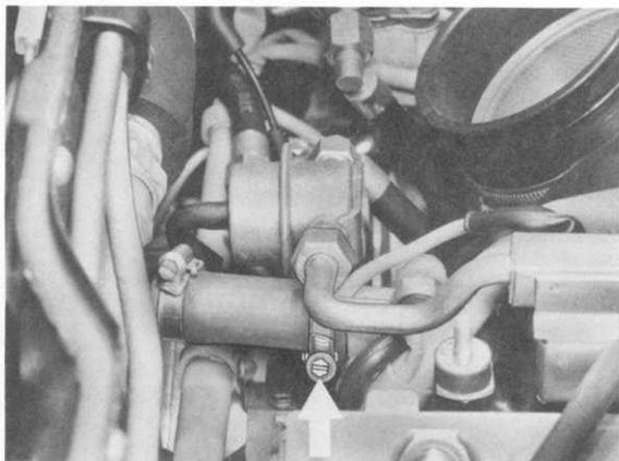
27. Disconnect air conditioner compressor plug connector, remove compressor from bracket and hang on one side with hoses in place.
