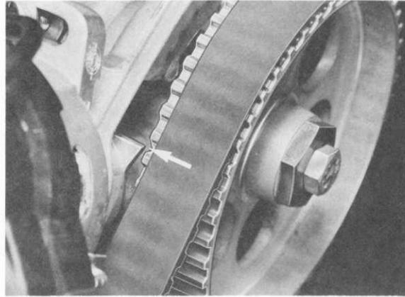
3. Install camshaft drive belt, always pre-loaded by hand, in the following order.
