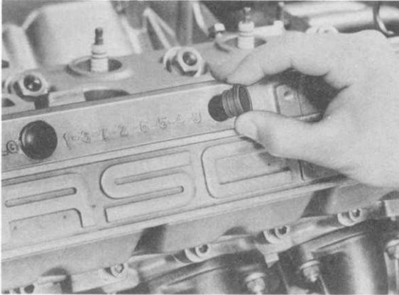
Lubricate plugs lightly and install by hand. For engine with aluminum plugs the torque is 40 Nm. Use new seals.
