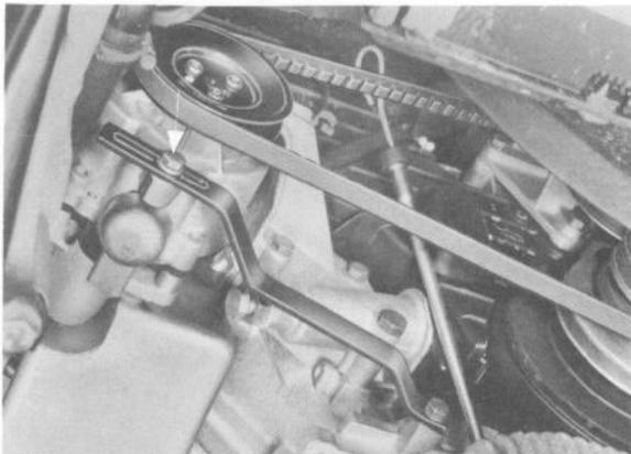
4. Loosen alternator bolt, swing alternator in (if necessary, detach alternator vent cover) and remove belt.
