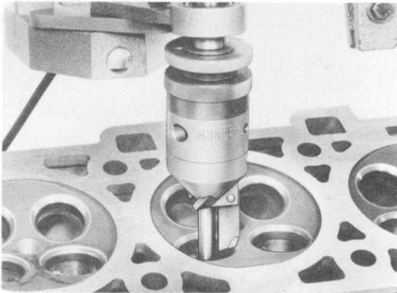
5. After the valve seats have been machined, use a grinding paste to lightly grind in valve seats. Check contact pattern of valve seat surface.
