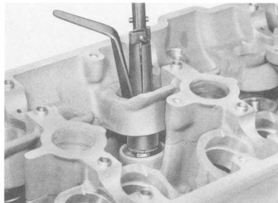
Oil valve stem and install valve. Push assembly sleeve over valve stem. Oil sealing lip of valve stem seal and position on assembly sleeve. Using Special Tool 9225/1 carefully and gently press seal onto valve guide until it is seated.
