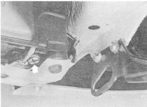
Remove water drain plugs on left and right side of crankcase.
