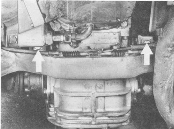
25. Disconnect and remove oil temperature sensor. Disconnect fuel return line while countering nut with second open-ended wrench.
