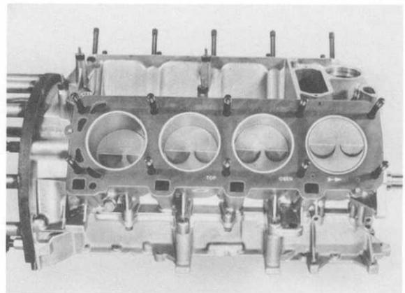
Position of installed cylinder head gasket. Watch marks, "TOP" and arrow, when installing. Arrow faces forward (see figure).
