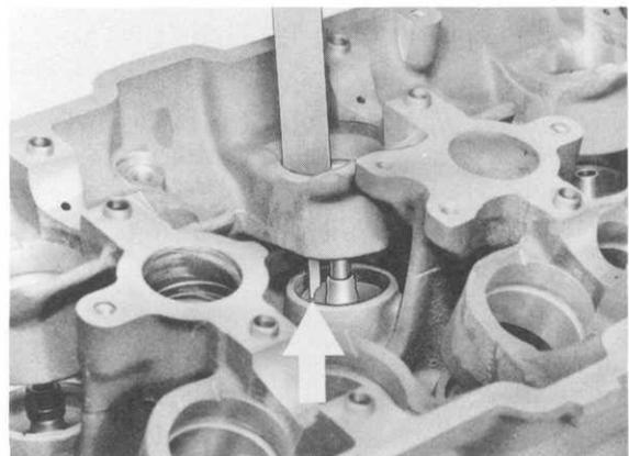
3. While measuring, hold the valve firmly against the valve seat.
