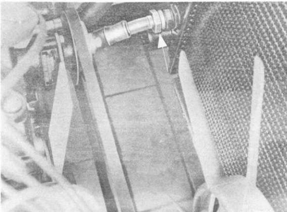
34. Remove engine mounts separately by applying a lifting force from one side to engine with a hydraulic jack, locally manufactured pad and an appropriate piece of wood on the oil pan, loosening the bolts, lifting the engine and removing the engine mounts.
