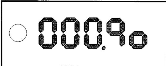
The function display will change to "r" after 10 000 ignition firings have elapsed.
