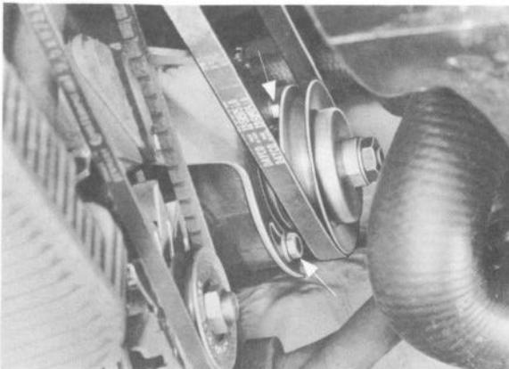
3. Loosen auxiliary air pump bolt, swing pump in and remove belt.
