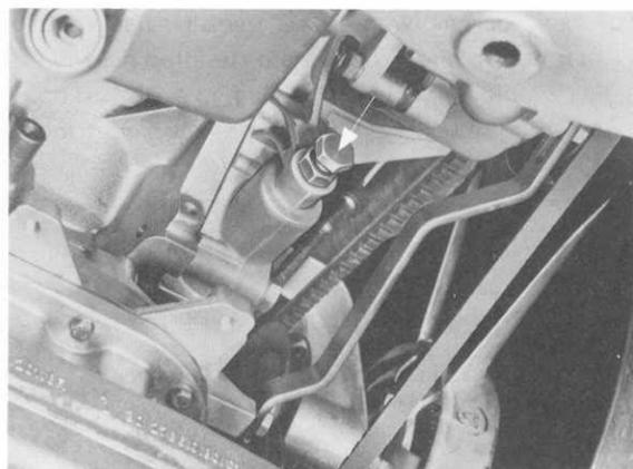
Loosen nut on adjusting screw and turn adjusting screw until the drive belt tightness is correct. Tighten nut again. Turn engine two more turns and recheck drive belt tightness.
