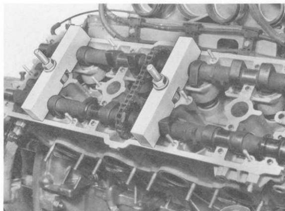
16. Install bearing bridges and bearing covers of camshafts. Bearing bridges and covers are machined with the cylinder head and must always be installed together. Note identifier and pairing code.
