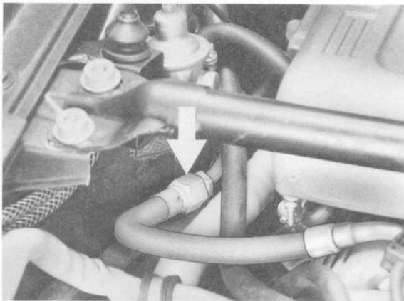
35. Disconnect ignition leads on both sides from distributor cover, remove both ignition coils from bracket and lay to one side.
