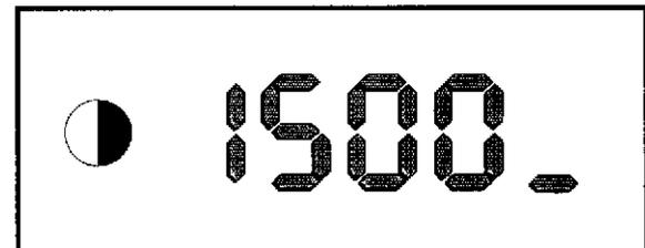
Press the *green* key until the clear symbol appears on the function display. The following display must then appear.
