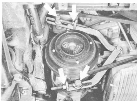
3. Unscrew lock nut and bolts on power pump, push in pump and take off drive belt.
