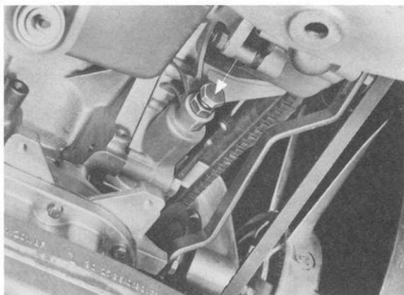
Loosen locknut of adjusting screw and turn adjusting screw until drive belt tightness is correct. Tighten locknut. Turn engine two turns and recheck tightness of drive belt.
