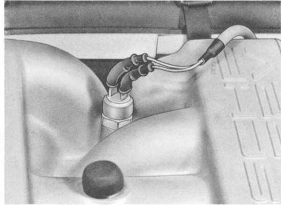
Tightening torque: 40 Nm (30 ftlb)
