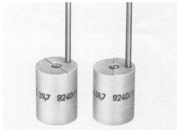
Measuring tools with installation length marked:
