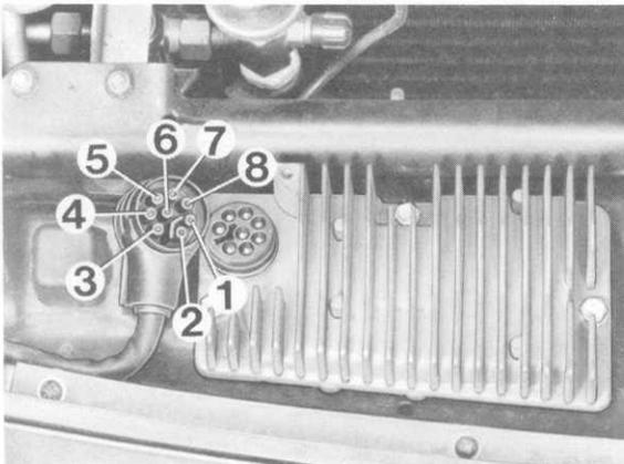
Connect voltmeter to pin 3 (ground) and pin 4 (plus) of the fan output-stage plug connector.
