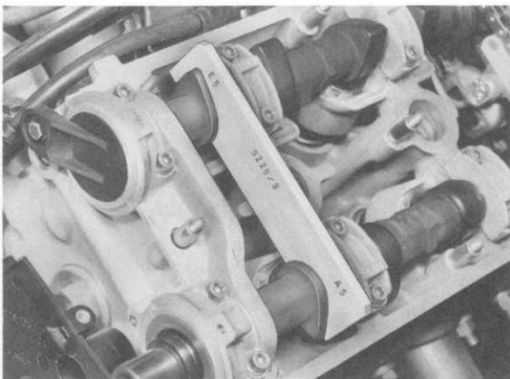
19. Use Special Tool assembly sleeve 9233 and pressure piece 9234 to drive in sealing ring on the camshaft input side. Oil sealing lip before assembly.
