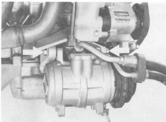
28. Detach both coolant hoses from cooler at regulator housing and remove.
