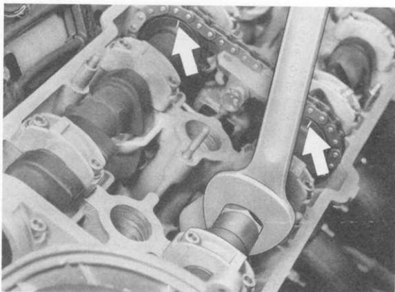
11. Unscrew and remove chain tensioner.
