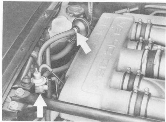
38. Disconnect underpressure hose from brake servo unit and remove.
