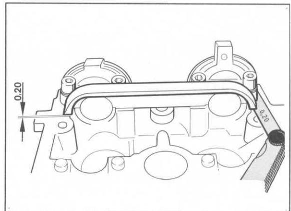
3. Apply a light film of oil to sealing cover and press on by hand. Tighten bearing bridge to specified torque.
