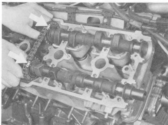
The distance between the markings on the inlet and outlet camshafts is 7 outer links of the chain, and/or approx. 113 mm spacing between the cast lugs.
