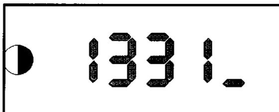
Operate the starter motor for approx. 5 seconds. The LED on the tester will go out shortly afterwards and the following display will appear.
