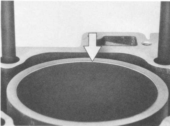
Before reassembly, thoroughly clean both halves of the crankcase so as to remove all trace of abrasive particles and silicone paste.
