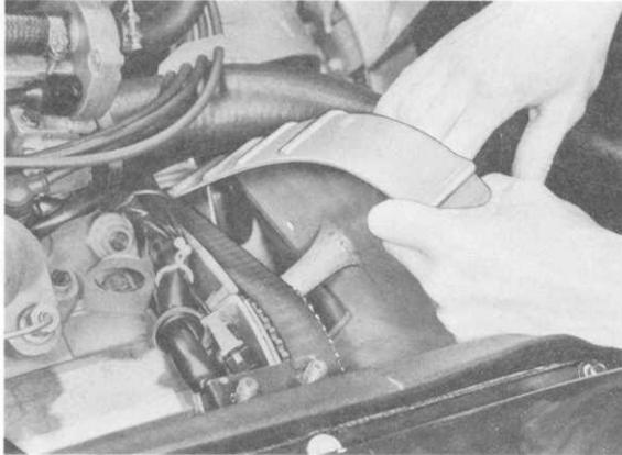
2. Turn engine in direction of rotation to TDC (cylinder 1). In this position marks on camshaft sprockets must be aligned with marks on flange bearings.
