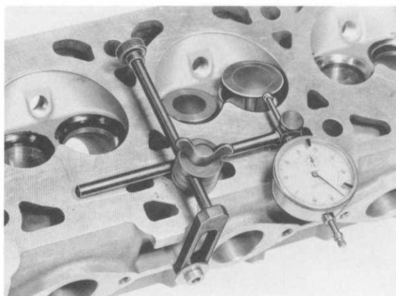
3. Check clearance with dial gage holder VW 387 and dial gage.
