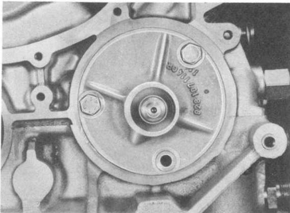
5. Tighten mounting nuts to final torque. See page 10 - 03 for specified torques and instructions.
