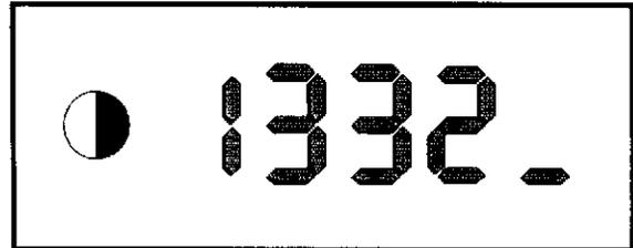
Press the accelerator pedal slightly. After approx. 20 mm, the LED must go out and the following display must appear.
