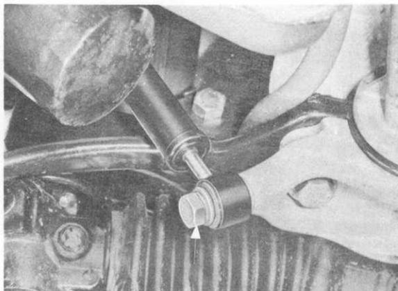
26. Detach engine shock absorbers with left and right mounts.
