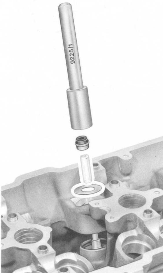
1. Oil valve stem and install valve. Place 1 mm thick washer on the cylinder-head mating face. Push assembly sleeve over valve stem. Oil sealing lip of valve stem seal and position on assembly sleeve. Using Special Tool 9225/1, push seal carefully and gently onto valve guide until seated.
