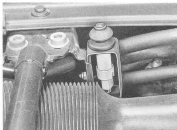
The output stage receives a square signal from the control unit. The output stage contains two mutually independent output-stage modules with separate protective circuits: each module controls a separate cooler fan.
