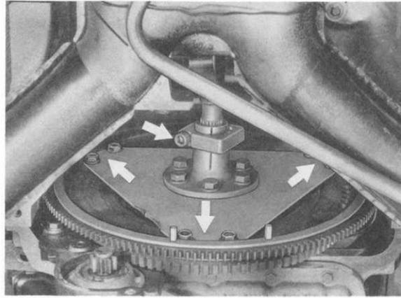
22. The pins for the oil temperature sensor must point downward before engine can be removed.
