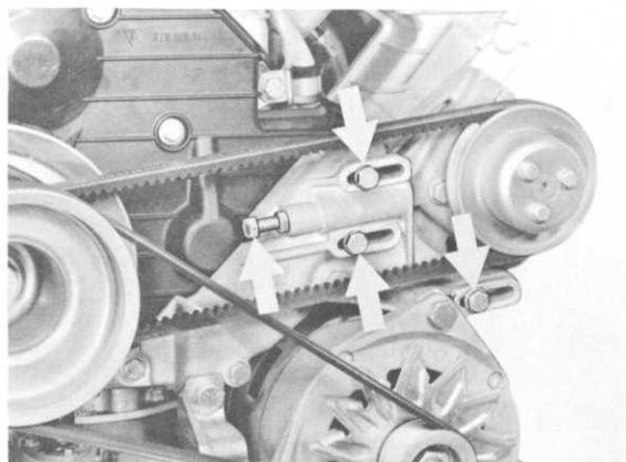
2. Unscrew both nuts and adjusting bolt for alternator. Swing in alternator, if necessary unscrew cowl, and take off polyrib drive belt.
