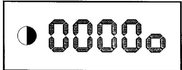
The error memory has been reset when the LED goes out and the function display changes to 0000.
