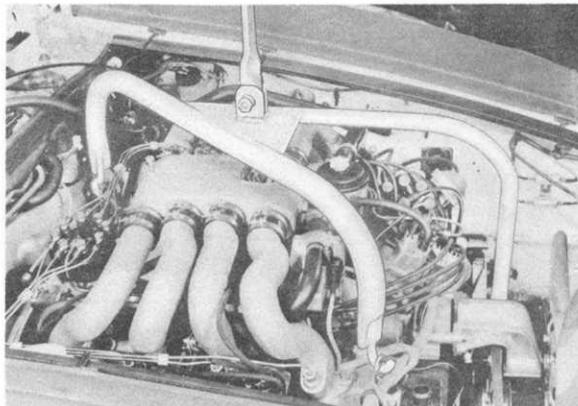
52. Unscrew top engine block/clutch housing mounting bolts.
