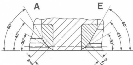
Valve seats may be machined down to the wear limit "A" = 14,5 mm (size new  $13.65 \pm 0.45$ ).
