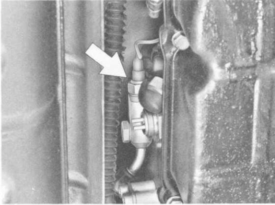
Tightening torque: 30 Nm (22 ftlb)
