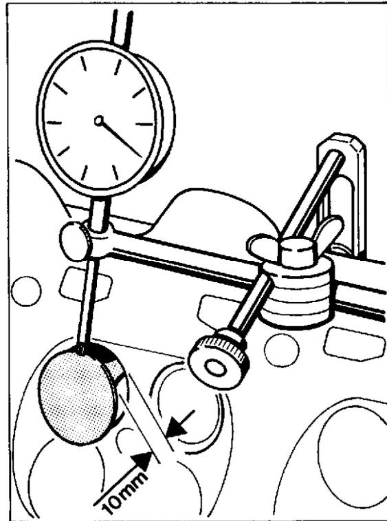
4. Measure rocker play at 10 mm valve lift (distance between valve head and valve seat). Wear limit for intake and exhaust valve guides = 0.80 mm.
