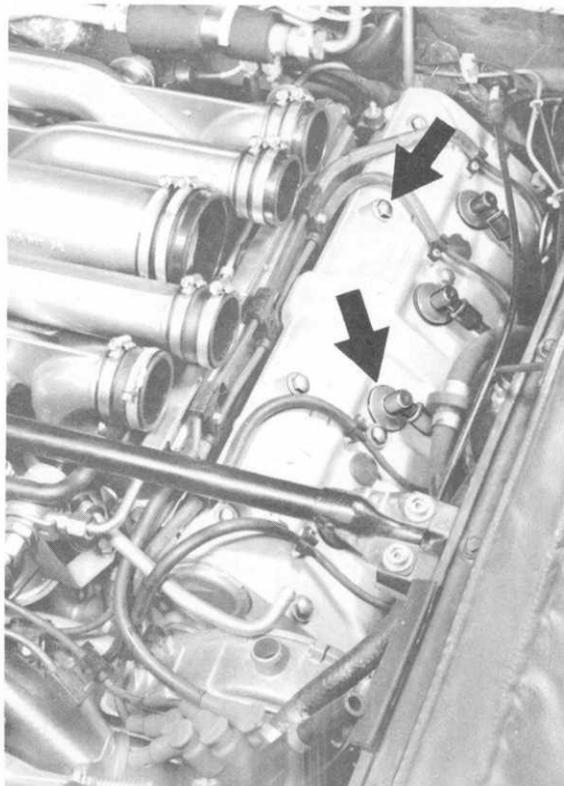
4. Unscrew suspension eye on engine only at rear left.
