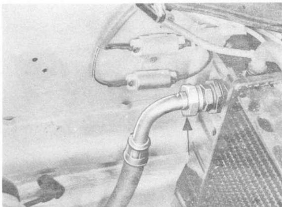
42. Disconnect B + wire, plug of transmitter wire to distributor and plug for engine wire harness.
